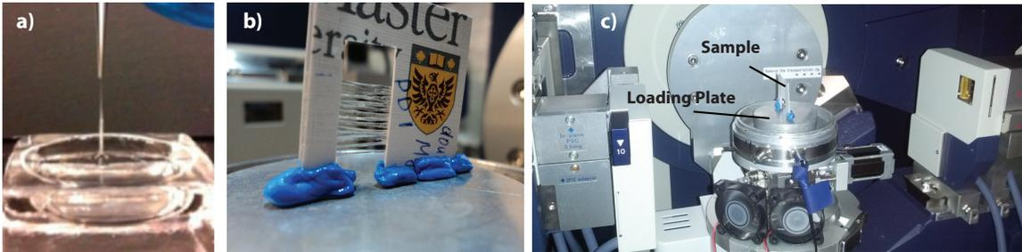
Figure 4.4: a) shows forceps drew from the surface of the solution into fibres. b) shows that fibres were taped horizontally on a cardboard. c) shows the setup of the X-ray experiment.
