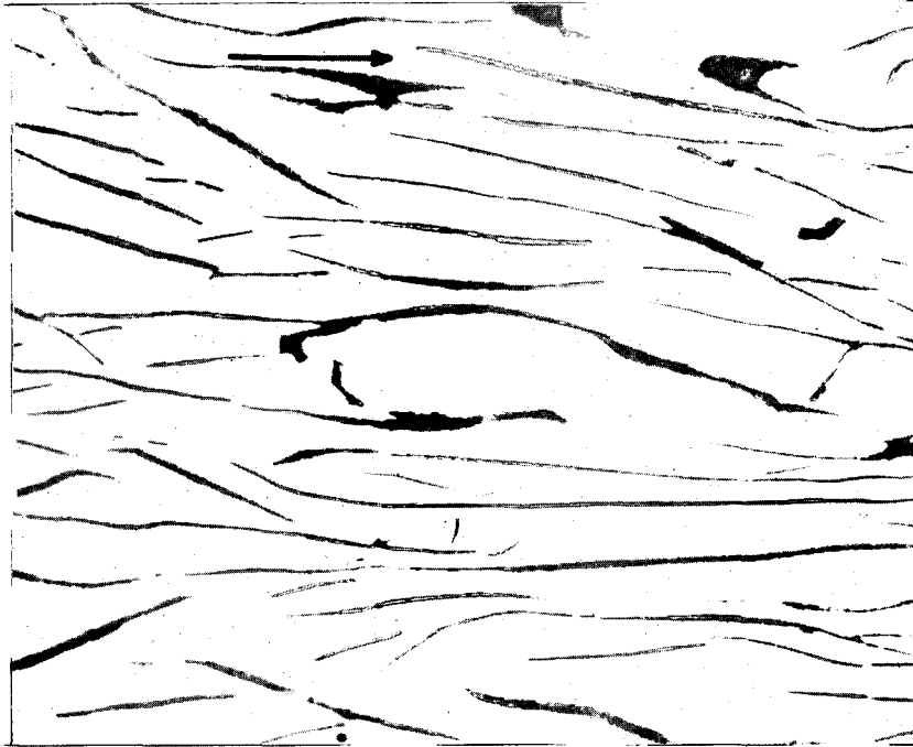
Figure 20 Micrograph of lamellar Fe-C alloy solidified at 2.0 mm/h. Arrow indicates the direction of solidification.(X83) (unetched)
