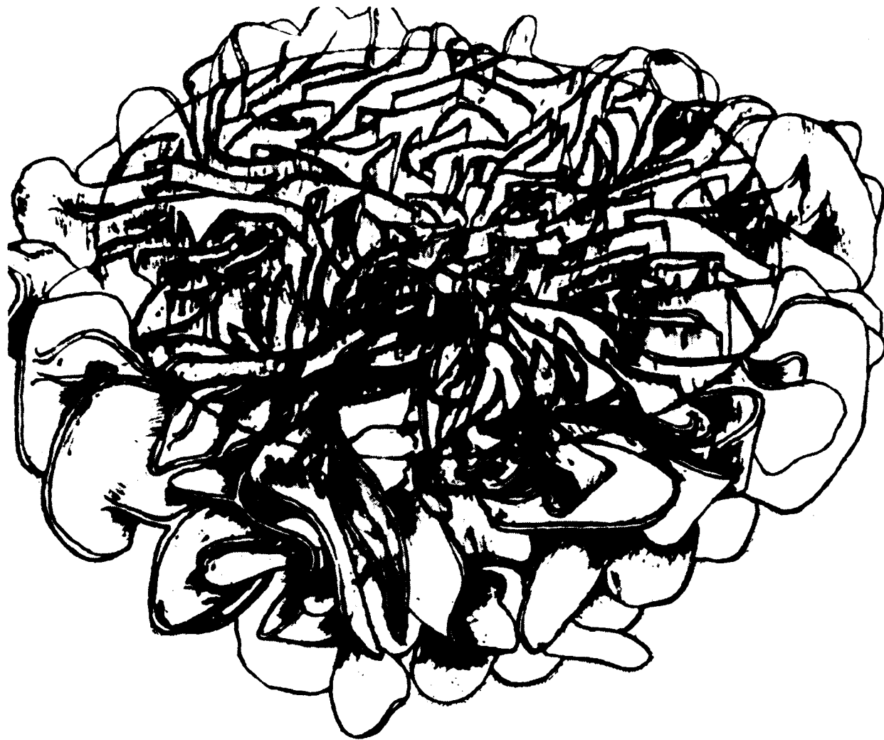
Figure 11 Artist's conception of the eutectic cell graphite structure.
