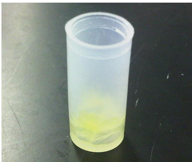
Fig. 53 Example of a polyethylene vial showing crystallized TPR-based boron sample material dried via dehydrator.
