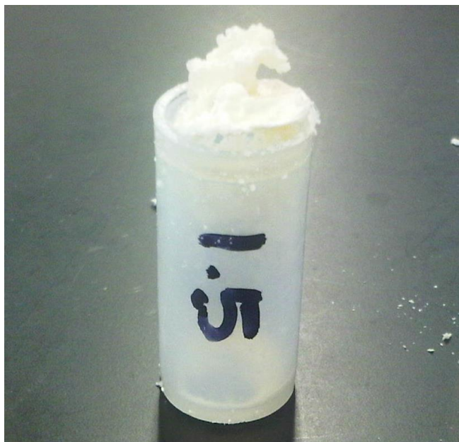
Fig. 49 Example of a polyethylene vial showing crystalline overgrowth of the lyophilized TPR-based boron sample material.
