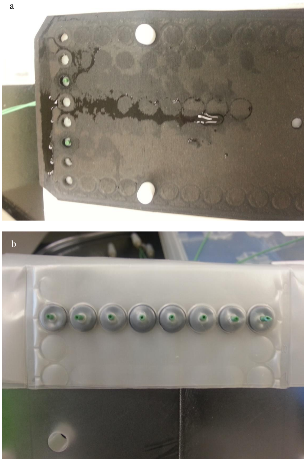
Figure 2.9. a. Leakage when using silicon rubber gasket. b. Custom made gasket composed of five Parafilm sheets, with silicone o-rings (5/16" OD) sandwiched between them.
