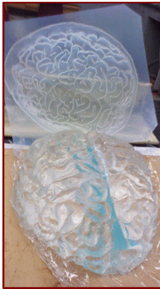
Figure 4.1: Silicone gel brain model after curing in a plastic brain mold
