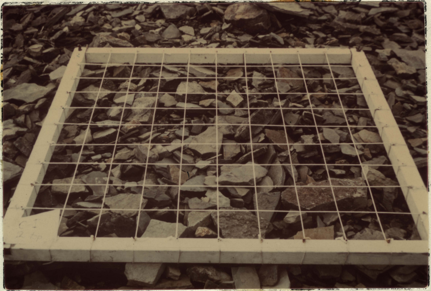
1. The one-metre square sampling grid.
