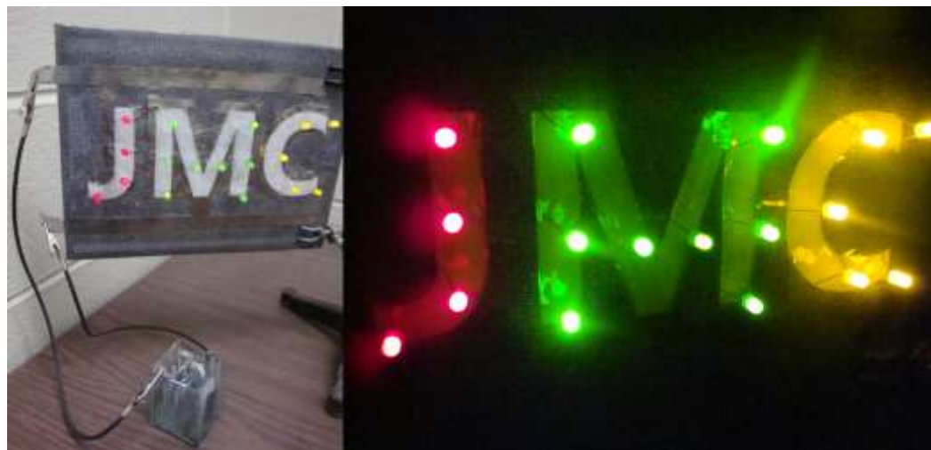
Figure 6-34 Seventeen LED bulbs powered by three envelop cells in series. The ES cell had an effective area of 6 cm 2 . Electrodes was prepared with ECR doped PPy/MWCNTs composite materials, with PPy/MWCNT mass ratio of 7:3. [177]
