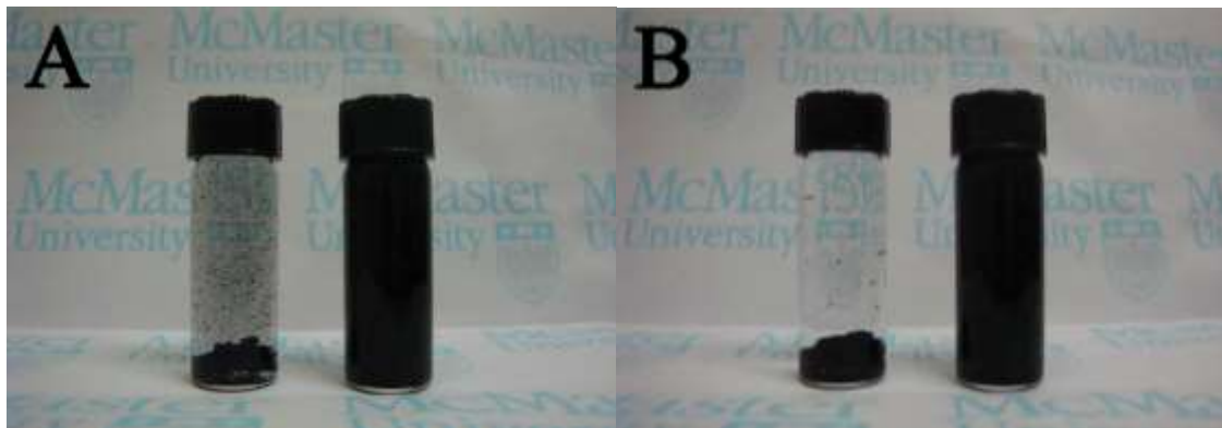
Figure 6-12 Comparative sedimentation tests of (left) MWCNT and (right) PPy/MWCNT composite materials with PPy/MWCNT mass ratio of 7:3, at same concentration in aqueous solution. Pictures of samples (A) as prepared and (B) after a week. [176]
