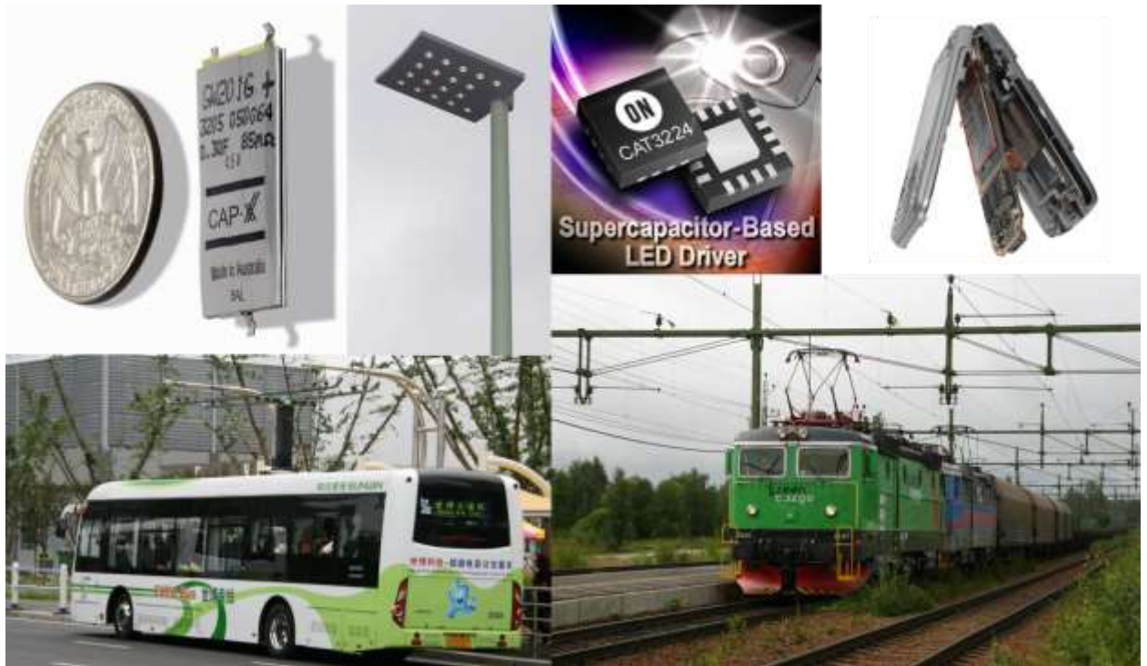
Figure 2-2 Application of ES devices: (First row) ES device, solar cell source with ES energy storage, ES based LED driver and corresponding cell phone; (Second row) ES based electric bus at 2010 Shanghai EXPO, Green Cargo from Bombardier Transportation.
