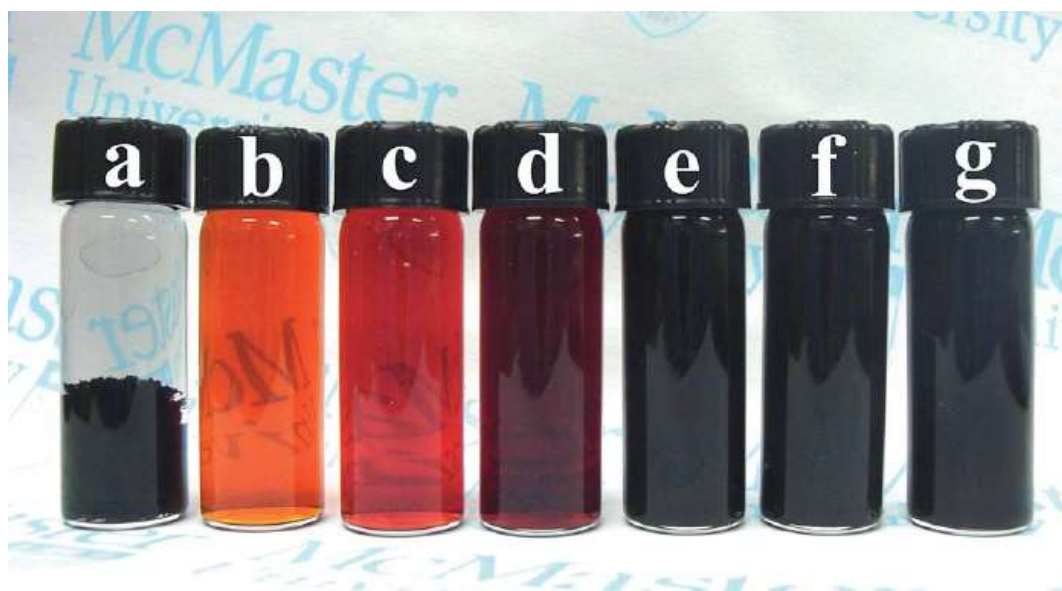
Figure 6-24 Dispersion performance test. (a) 1 g L -1 MWCNT in water, (b) 1 g L -1 PV aqueous solution, (c) 1 g L -1 ECR aqueous solution, (d) 1 g L -1 AF aqueous solution, (e) 1 g L -1 MWCNT in 1 g L -1 PV aqueous solution, (f) 1 g L -1 MWCNT in 1 g L -1 ECR aqueous solution, and (g) 1 g L -1 MWCNT in 1 g L -1 AF aqueous solution. Suspensions (e-g) stable for 3 months. [177]
