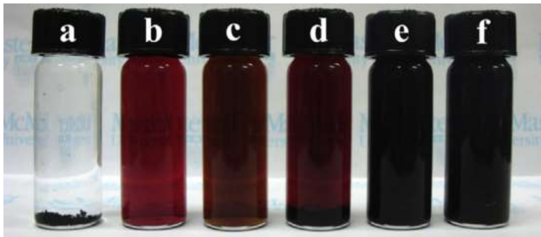
Figure 6-10 Dispersion performance test. (a) 1 g L -1 MWCNT in water, (b) 1 g L -1 amaranth aqueous solution, (c) 1 g L -1 PV aqueous solution, (d) 1 g L -1 MWCNT in 1 g L -1 amaranth aqueous solution, (e) 1 g L -1 MWCNT in 1 g L -1 PV aqueous solution, and (f) 1 g L -1 MWCNT in aqueous solution, containing 1 g L -1 amaranth and 1 g L -1 PV. [176]
