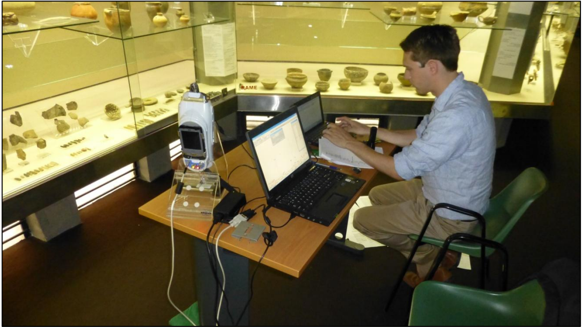
Figure 5.2 A Bruker Tracer III-SD portable XRF machine in use at the Paolo Orsi Archaeological Museum in Syracuse, Sicily.
