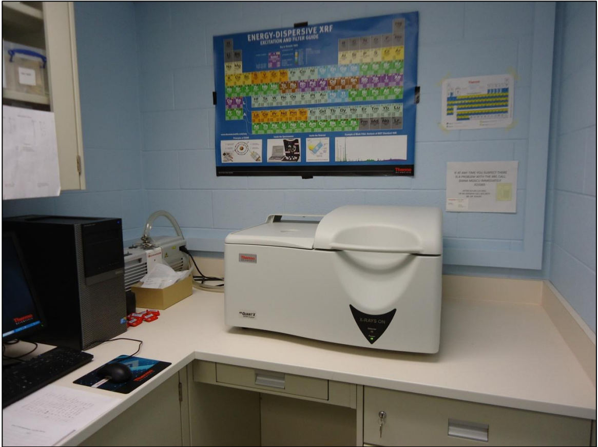
Figure 5.3 A Thermo Scientific ARL Quant'X EDXRF spectrometer used to analyze artifacts from the Italian island of Sardinia.
