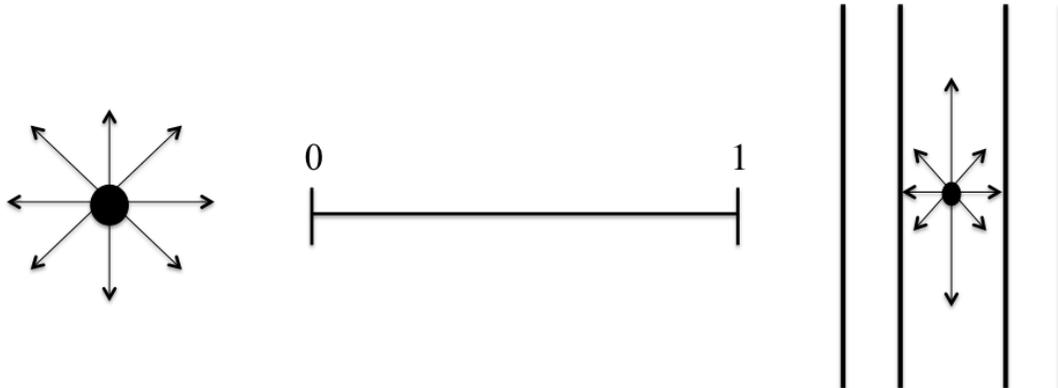
**Figure 1.4: Schematic representation of the meaning of fractional anisotropy (FA) values.** FA values scaling closer to zero, as illustrated on the left, represent a spherical shape since diffusion would be of the equal magnitude in all directions. Values approaching 1 represent the diffusion primarily in one direction, as in the hypothetical case of an infinitely long cylinder.
