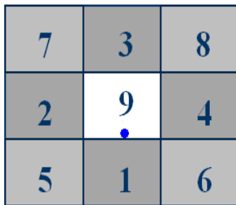
Figure 3.15 Configuration of the 4\pi NaI(Tl) detector assembly and placement of point source
