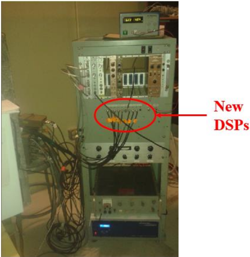
Figure 2.5: Digital Processing Systems Configuration for the 4\pi Nine NaI(Tl) Detector Array
