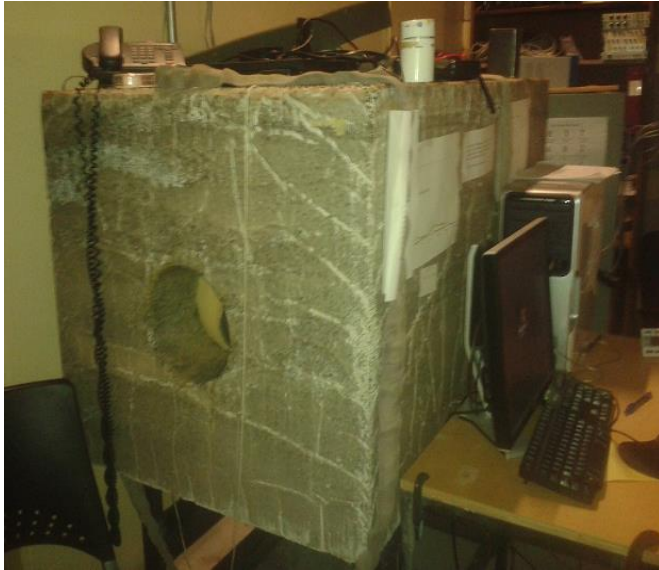
Figure 2.3: McMaster University 4\pi NaI(Tl) gamma-ray detector array
