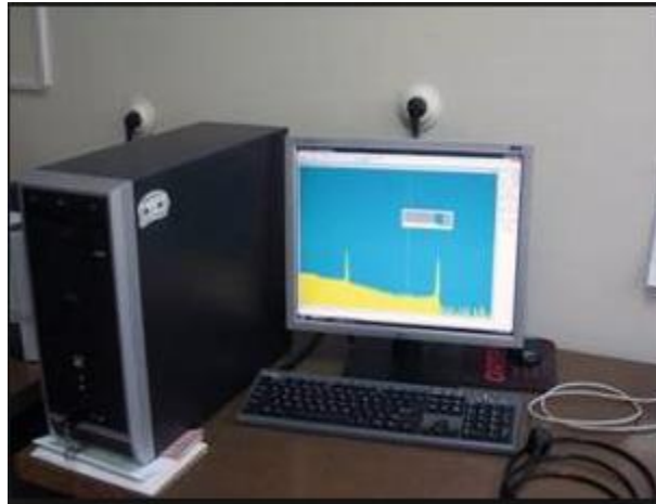
Figure 2.8: ORTEC GammaVision 32 software used for spectrum acquisition and on-line analysis
