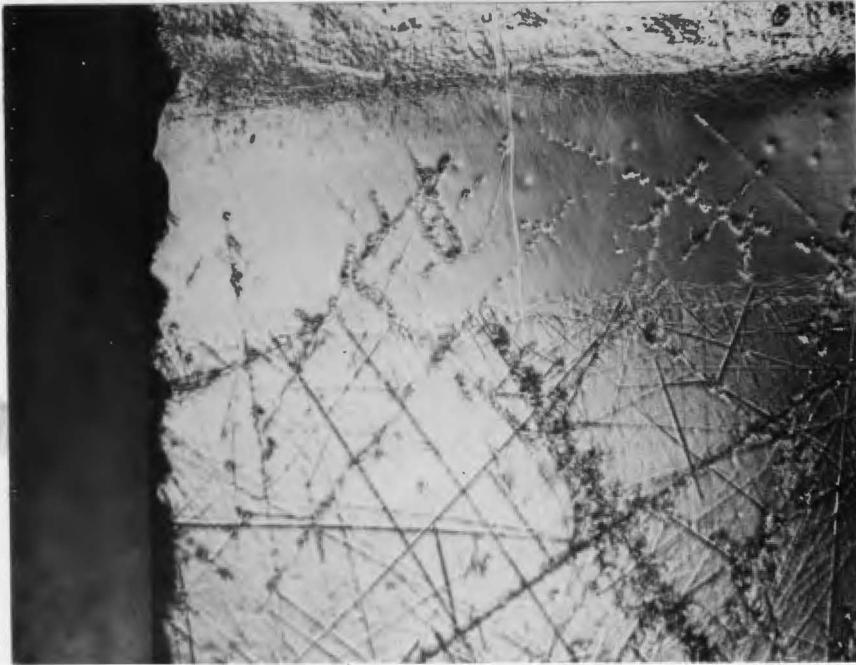
Fig. 3: Single-layer wafer, lapped at 3^\circ and etched in 3 \text{ H}_2\text{O} : 1 \text{ HNO}_3 . Layer thickness \approx 22\mu .
