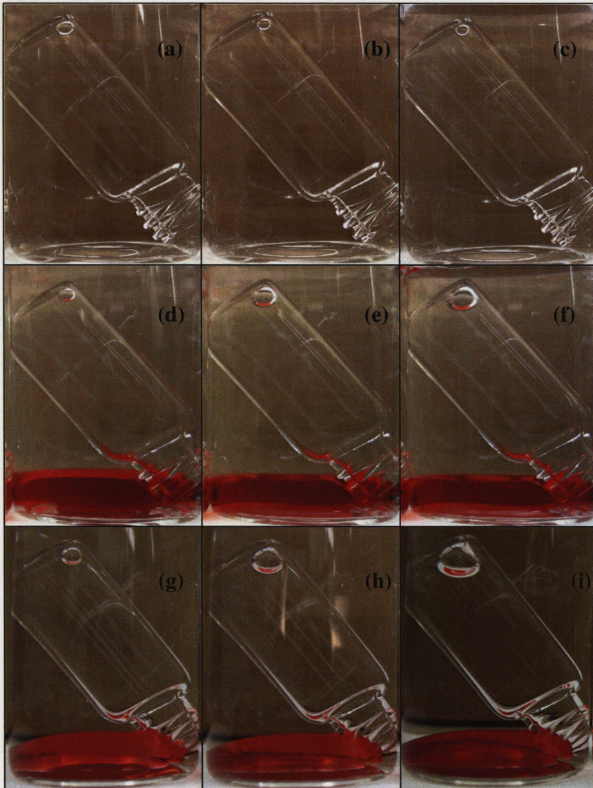
Figure 2.3. Images of control experiments at (a) 0 days, (b) 124 days, and (c) 215 days; PCE experiments at (d) 0 days, (e) 124 days, and (f) 215 days; and tDCE experiments at (g) 0 days, (h) 10 days, and (i) 22 days. Note that the red colour observed on the bottom shoulder of the inner vial and the lower surface of the gas bubble in the PCE and tDCE experiments is caused by reflection from the dyed NAPL pool and is not indicative of NAPL on these surfaces.
