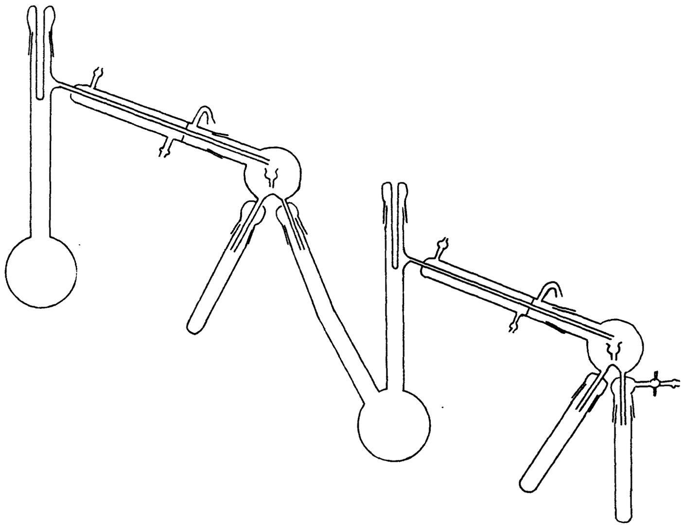
Fig. 2 FLUOROSULPHURIC ACID DISTILLATION APPARATUS
