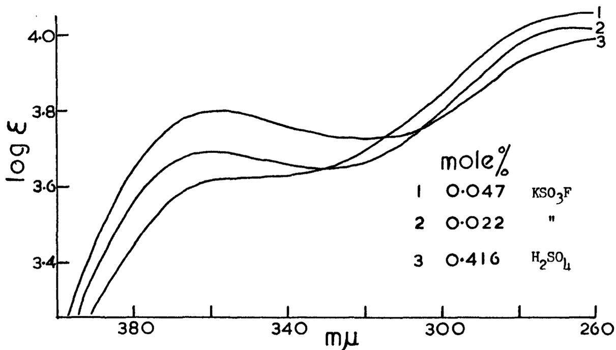
Fig. 37 SOLUTIONS OF 1-CHLORO-2,4-DINITROBENZENE: ABSORPTION SPECTRA.
