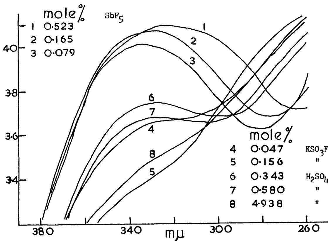
Fig. 36 SOLUTIONS OF 1-FLUORO-2,4-DINITROBENZENE: ABSORPTION SPECTRA.
