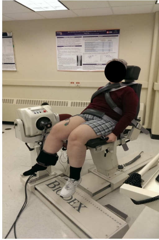
Figure 4.13. System 2 dynamometer setup for measuring knee extension and flexion MVIC and isokinetic torque in legs with symptomatic, radiographic knee OA (Biodex, NY).
