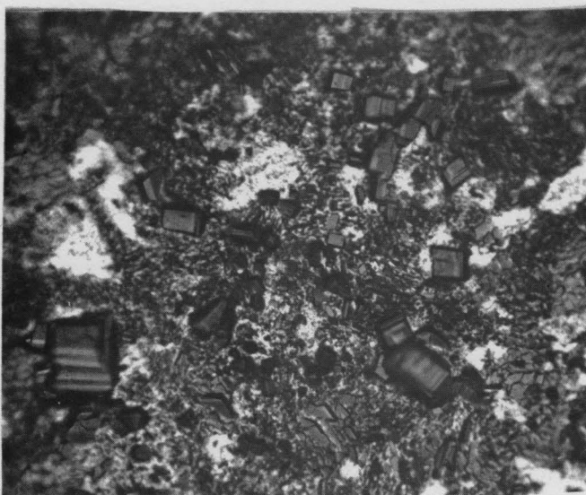
Figure 5-(30) Fe - 1.065%C X530 10 min. in pure CO 2 Topography of Specimen showing Oxide Growth Centres and Oxide Coverage
