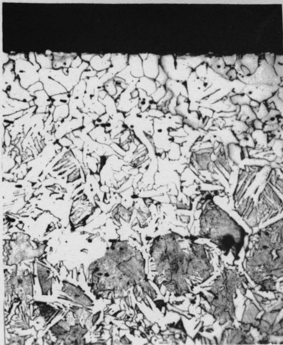
Figure 5-(35) Fe - 1.065%C X250 75 min. in \frac{60}{40} = \frac{CO_2}{CO} Structure of Decarburized Alloy
