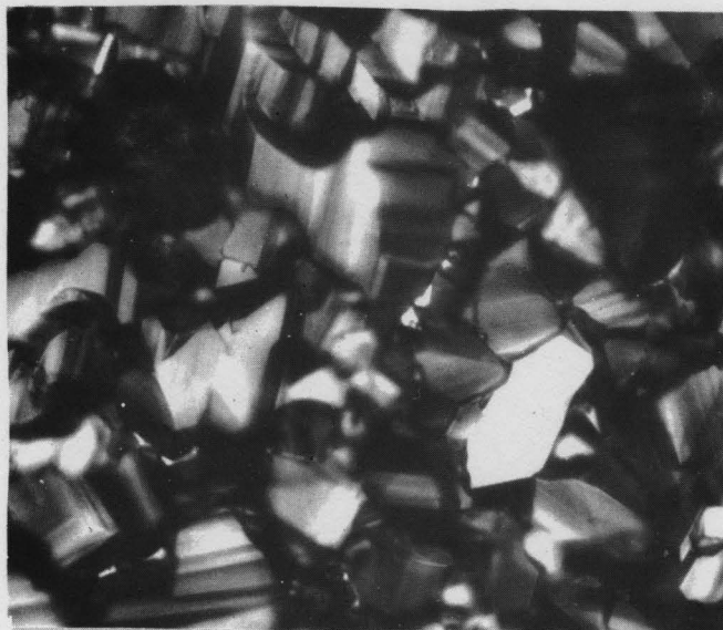
Figure 5-(19) Fe - 1.065%C X700 20 min. in \frac{60}{40} = \frac{CO_2}{CO} Impingement of crystallite boundaries
