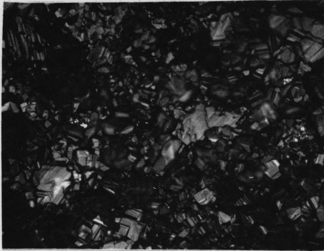
Figure 5-(31) Fe - 1.065%C X530 30 min. in pure CO 2 Surface Oxide Coverage
