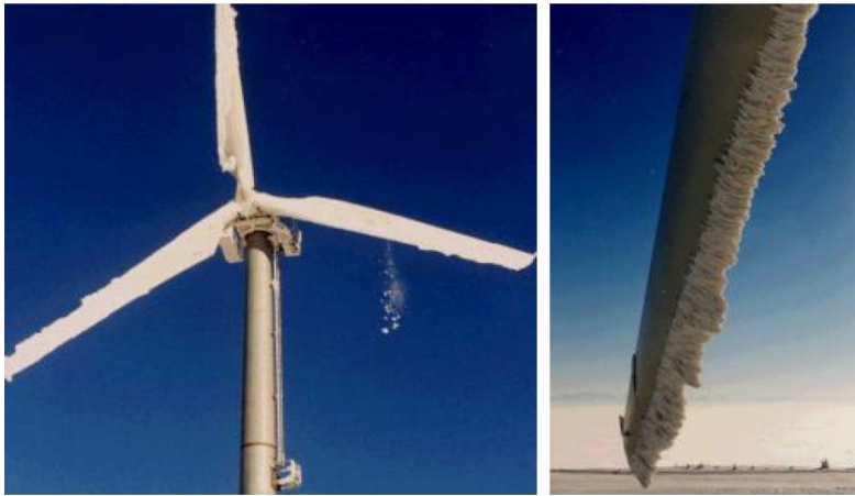
Figure 2.4: Rime ice formation on the leading edge of a 150 kW wind turbine blade, Grenchenberg, Switzerland [5]
