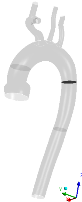
Figure 26: Orientation of aorta for simulations with ascending aorta, descending aortic arch and descending aorta planes shown.
