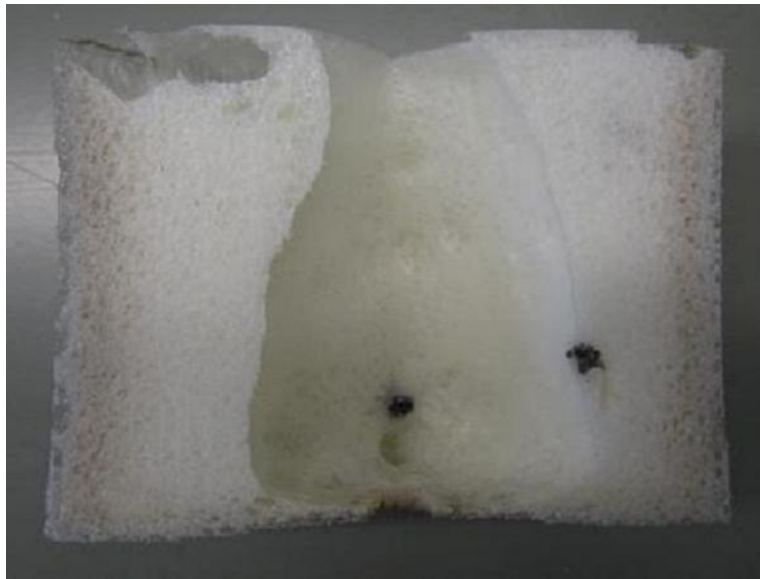
Figure 5-7: PE-1 + 2.5% CBA- Monolayer foam with extensive structural failure.
