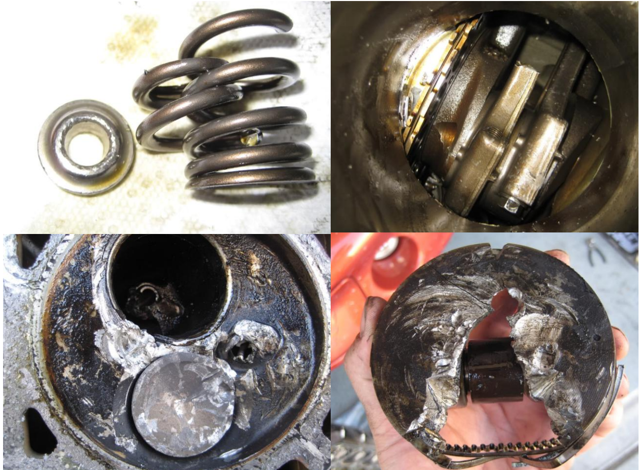
Figure 3-6: Catastrophic engine failure (Top left: Broken spring, Top Right: Broken con-rod, Bottom left: Damaged cylinder head, Bottom Right: Damaged piston)
