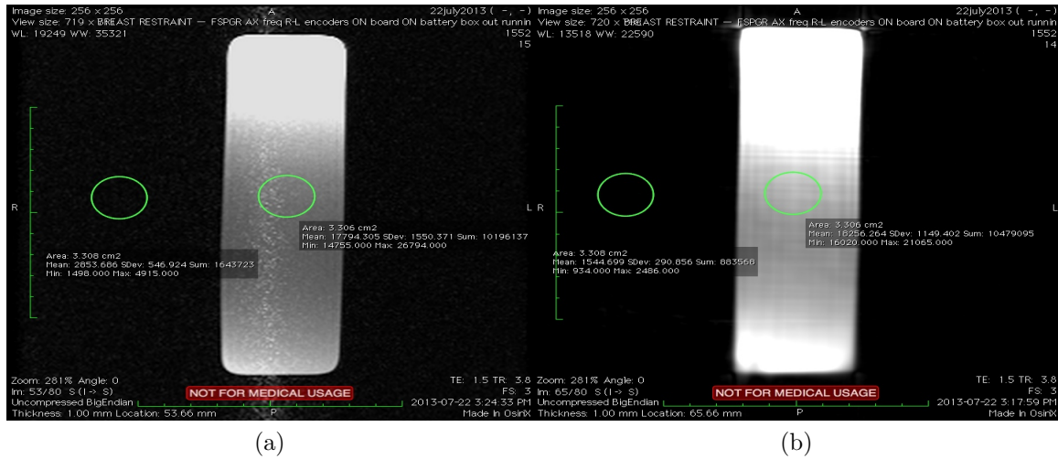
Figure 5.9: MR images acquired in the presence of stabilization device: a) device moving. b) device moving with lower imager receiver gain. The green circles represent the regions of the image used in the calculation of the SNR.
