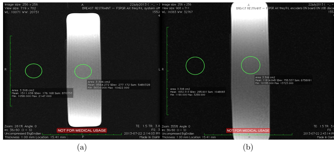
Figure 5.8: MR images acquired in presence of the stabilization device. a) encoders are powered off. b) encoders are powered on. The green circles represent the regions of the image used in the calculation of the SNR.
