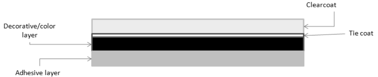
Figure 1-2: Typical construction seen in a automotive-grade multilayer decorative film
