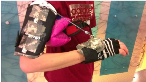
Figure 1: Device showing highest flexion setting
