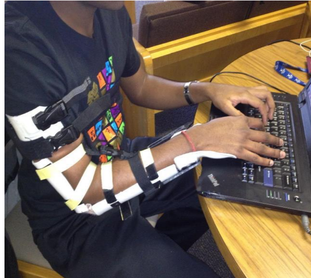
User typing with the help of Elbow Flex.
