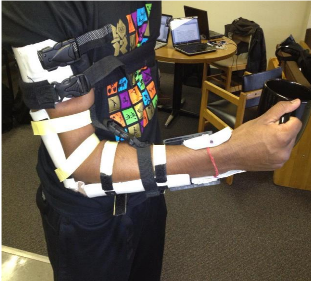
User holding object at a flexed position with the help of Elbow Flex
