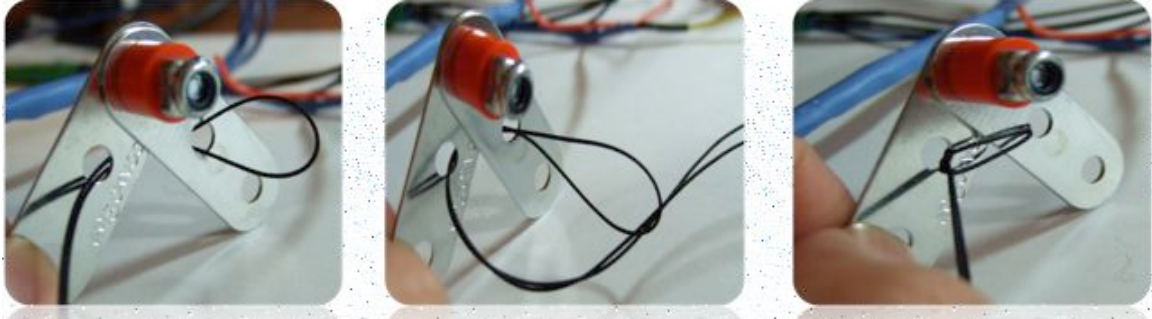
Figure 24 - Cable Loop Forming Procedure
