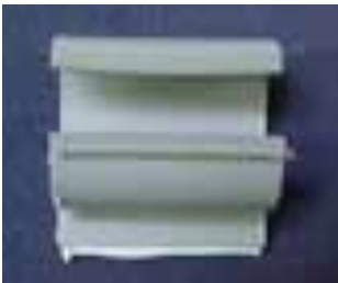
Figure 25 - Plastic Motor Clip Holder Used to Hold Solenoid
