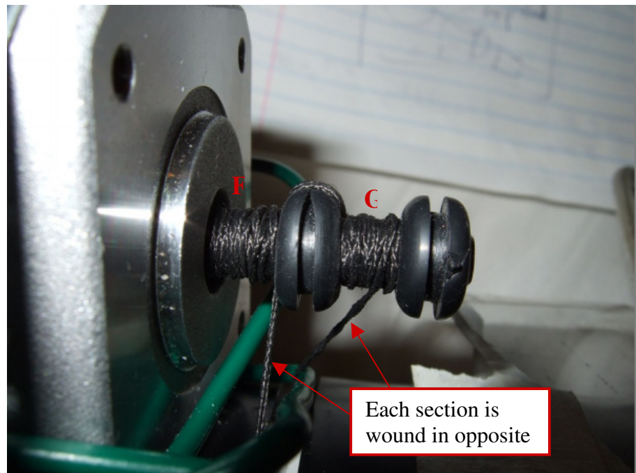
Figure 14 – Photograph showing bidirectional winch system on motor shaft
