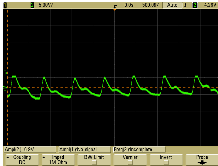
Figure 25: PPG signal acquired from passive filtering
