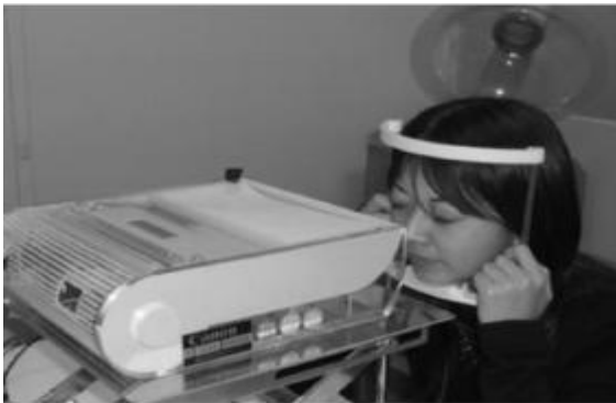
Figure 2.4- Inkjet Delivery System
