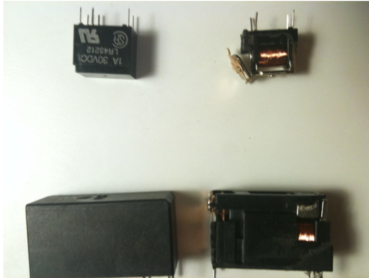
Figure 21 – Relays side by side
