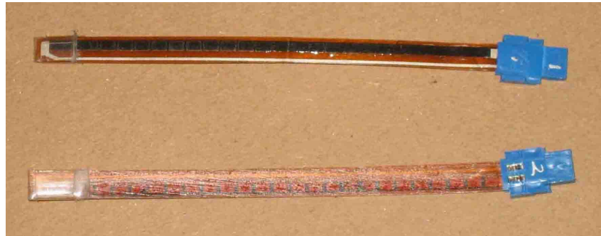
Figure 4.1; Bi-directional flexible bend sensors used for the project
