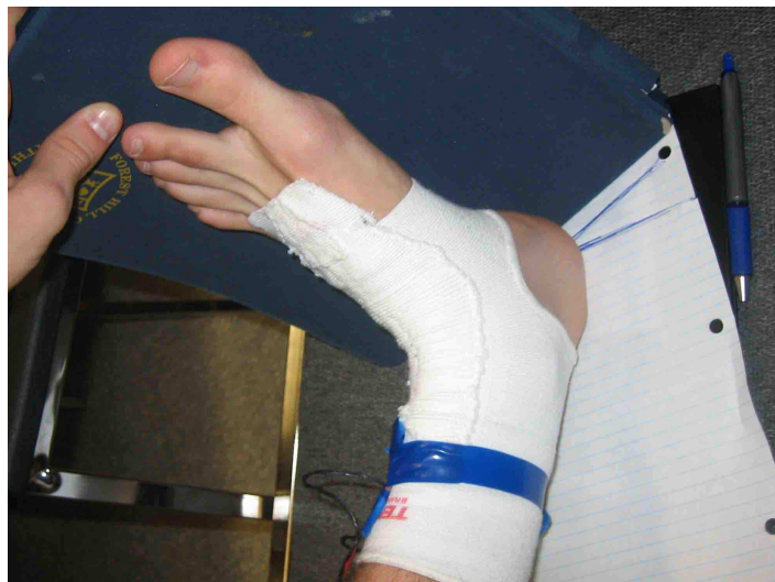
Figure 4.4; Calibration of IE sensor. Angle is measured using protractor on intersecting lines on the paper
