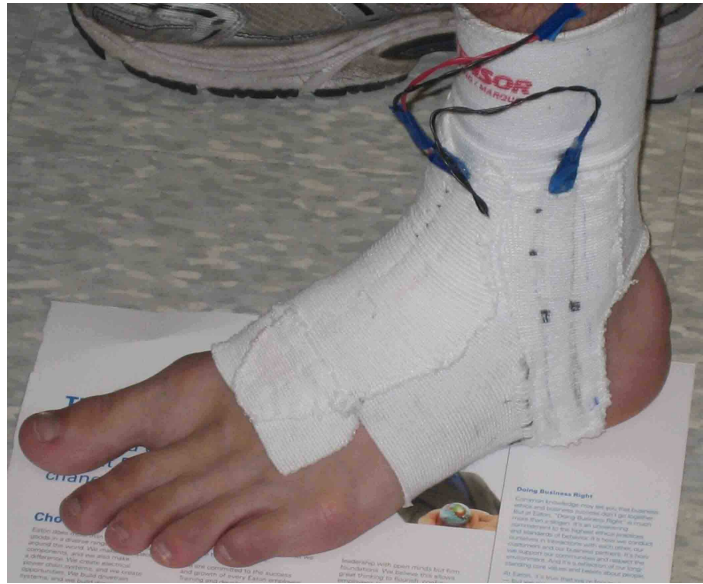
Figure 4.6; Ankle sleeve prototype with sensors embedded on the lateral and anterior sides
