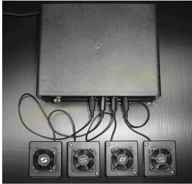
Figure 2.2: Hardware device used to deliver olfactory stimulus in the SUBSMELL system.
