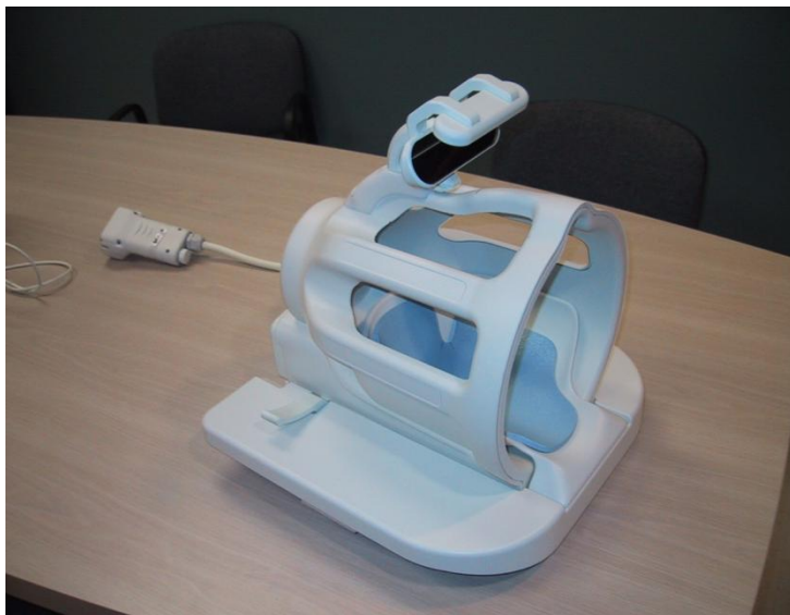
Figure 3.1: Head coil used for data acquisition during the fMRI protocol.
