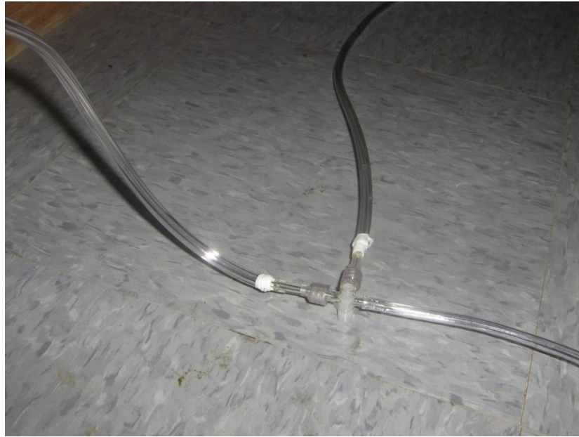
Figure 4.3: Manually operated three way control valve used to direct medical air in two directions. During stimulus presentation the air is passed through the nebulizer and during non-stimulus periods, the air flow passes directly to the subject.
