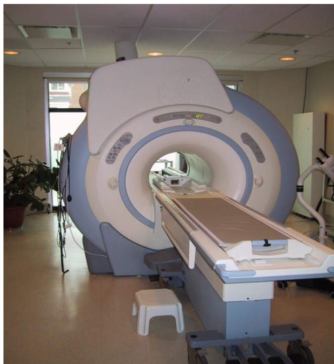
Figure 3.2: 3T GE short bore MRI machine used for performing the fMRI experiments.
