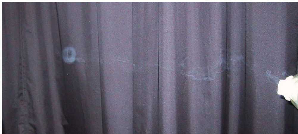
Figure 2.3: Demonstration of the creation of a vortex ring by means of a rubber bladder impacted by solenoids to force smoke through a small aperture.
