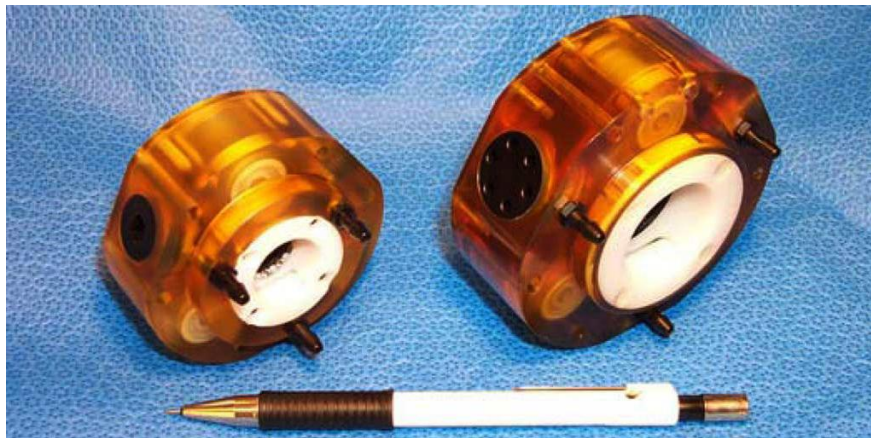
Figure 2.6: Final design of the PneuStep pneumatic stepping motor in two different sizes. All parts are MRI compatible. Note the three input nozzles for compressed air control.
