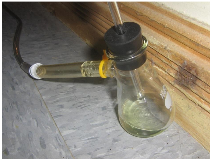
Figure 4.2: Homemade nebulizer used to convert a scented liquid into a vapour for presentation to the subject during the fMRI experimental trials.
