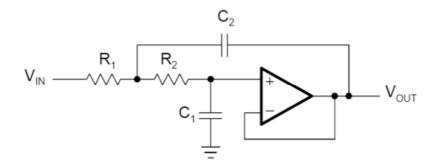
Figure 6 - Low pass filter configuration for -15V to +15V rails
