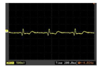
Figure 10 - ECG produced using 2 standard Ag AgCl electrodes directly on the skin
