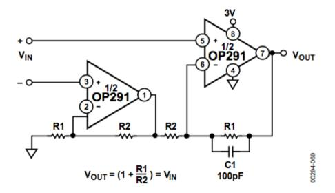
Figure 8 - Single 3V Supply Instrumentation Amplifier
