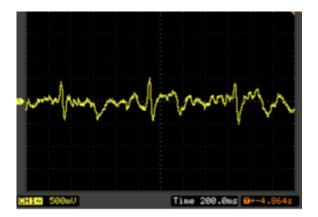
Figure 11 - Example ECG with held breath using the capacitively coupled electrodes through a standard cotton T-shirt
