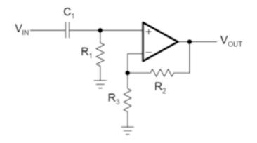
Figure 4 - High pass filter configuration for -15V to +15V rails
