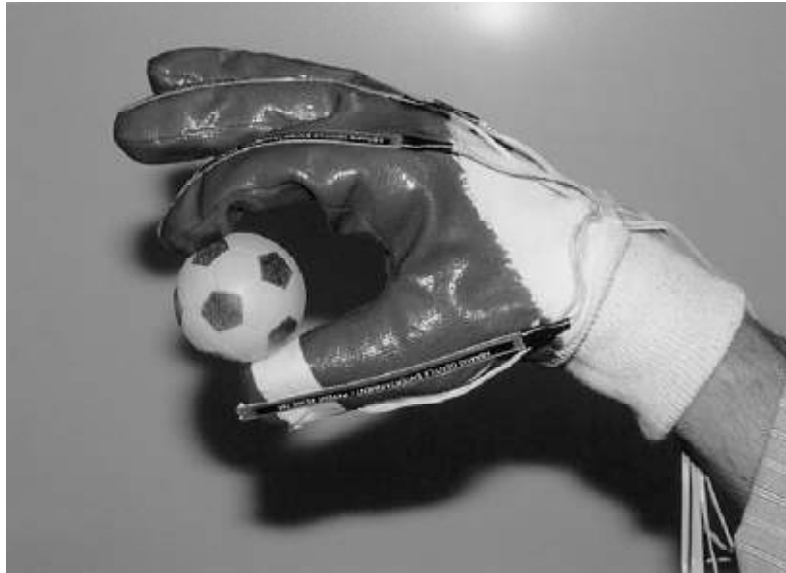
Figure 2.1: Prototype Data Glove. Flex sensors mounted on the glove and white coloured force sensor taped around thumb.
