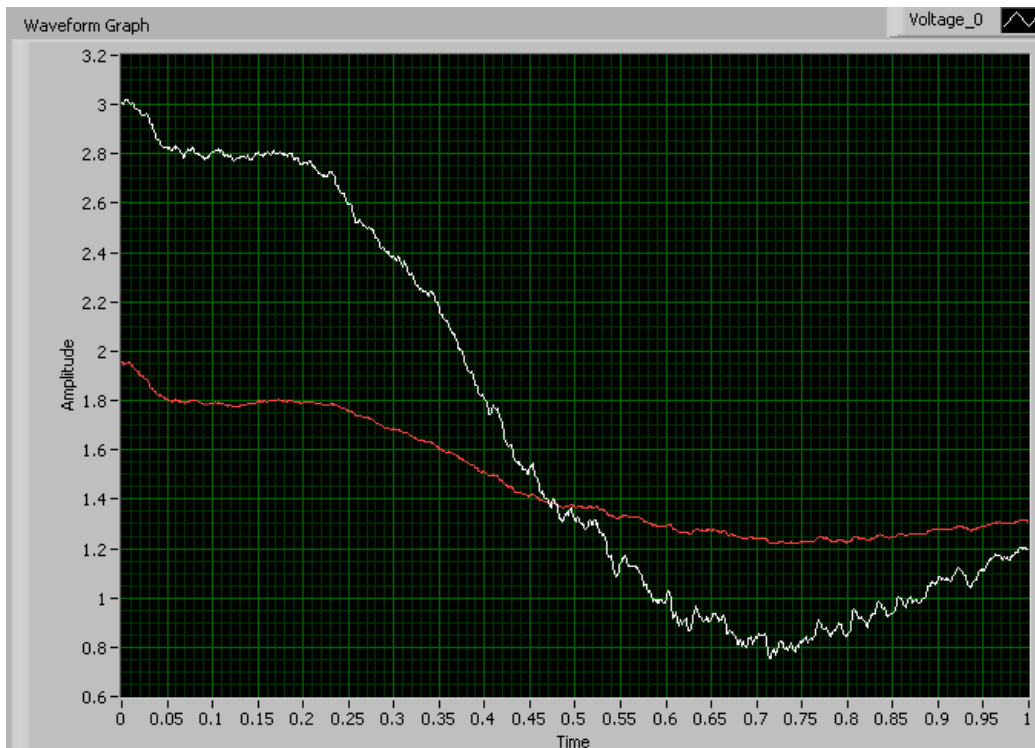
Figure 5.4: This shows the extension of the fingers. As the fingers are extended, the voltage response decreases.
