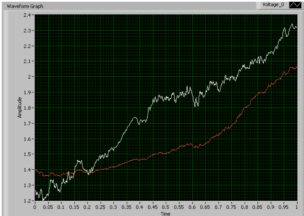
Figure 5.3: This picture shows flexion of the fingers. As seen in the graph, when the fingers are flexed, the voltages increase and the graphs move upward. (the top line is thumb and the bottom one is index)
