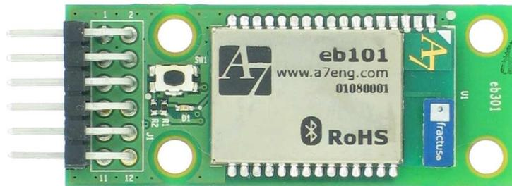
**Figure A.7:** eb301 Bluetooth module used for the NIHMS<sup>13</sup>.
