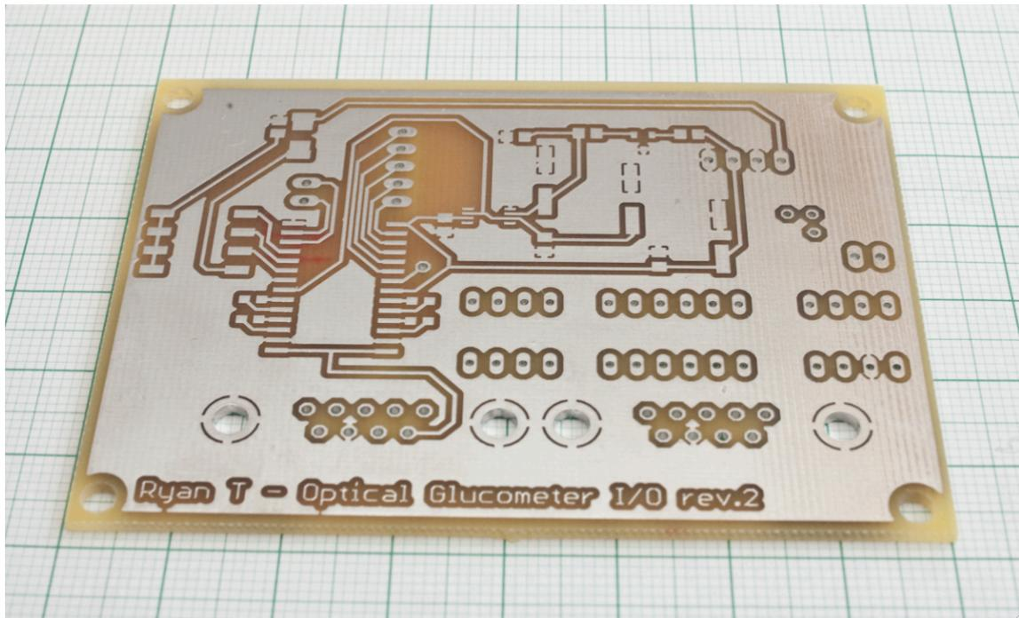
Figure 9: PCB Top side
