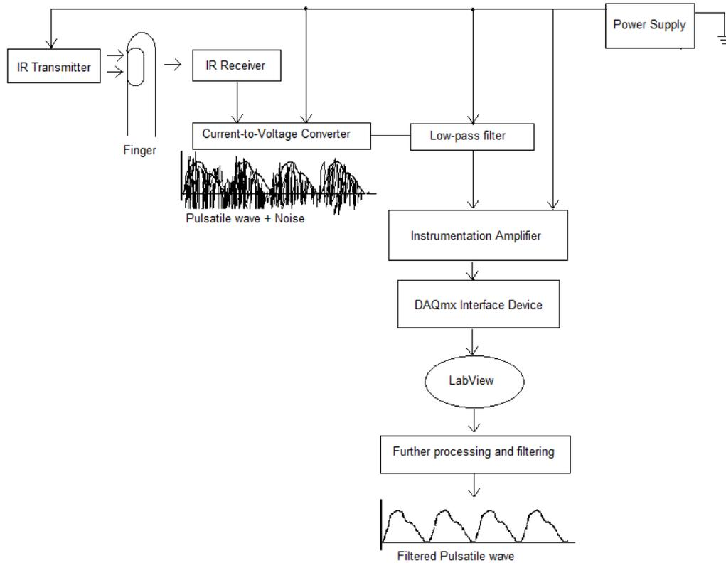
Figure 20: Block Diagram of the Pulse Oximeter
