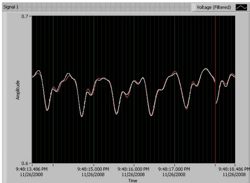
Figure 18: Processed signal from rudimentary Pulse Oximeter.
