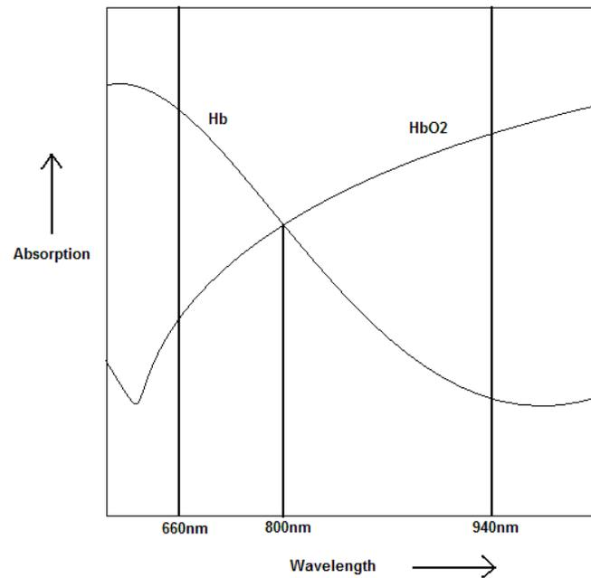
**Figure 19: Absorption spectrum of HbO<sub>2</sub> and Hb over a wavelength of 500-1000nm**
