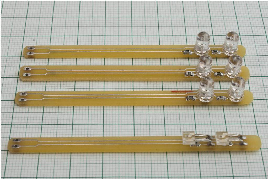
**Figure 1: Source assemblies: from top to bottom: 1550nm, 1400nm, 1300nm and 940nm.**
