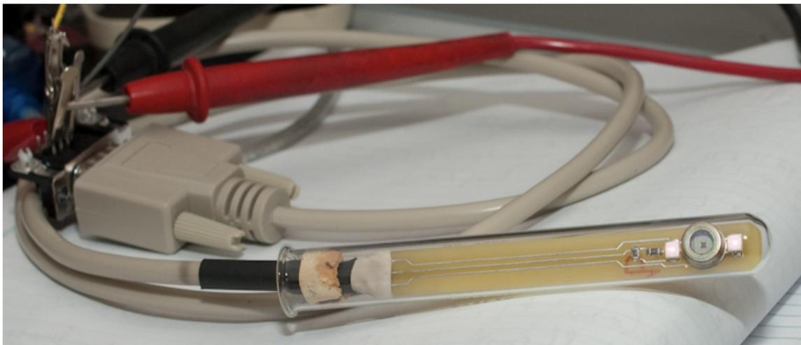
**Figure 3: Detector Assembly (Dual-Mode) in test tube wired to a Serial cable.**
