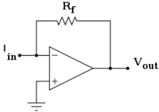
Figure 21: Current to Voltage Converter
