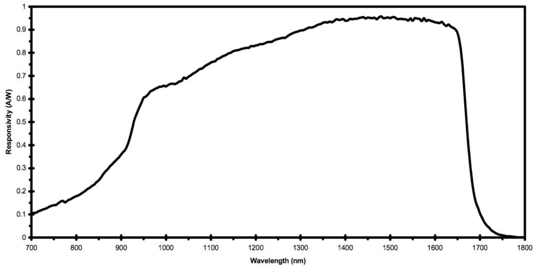
**Typical Responsivity Curve using Thorlabs calibration services.**
