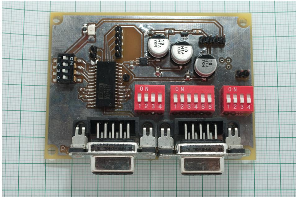
**Figure 16: Completed Glucometer Interface Board**
