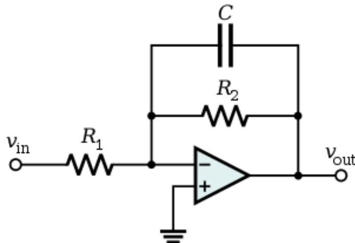
Figure 22: Active Low-Pass Filter
