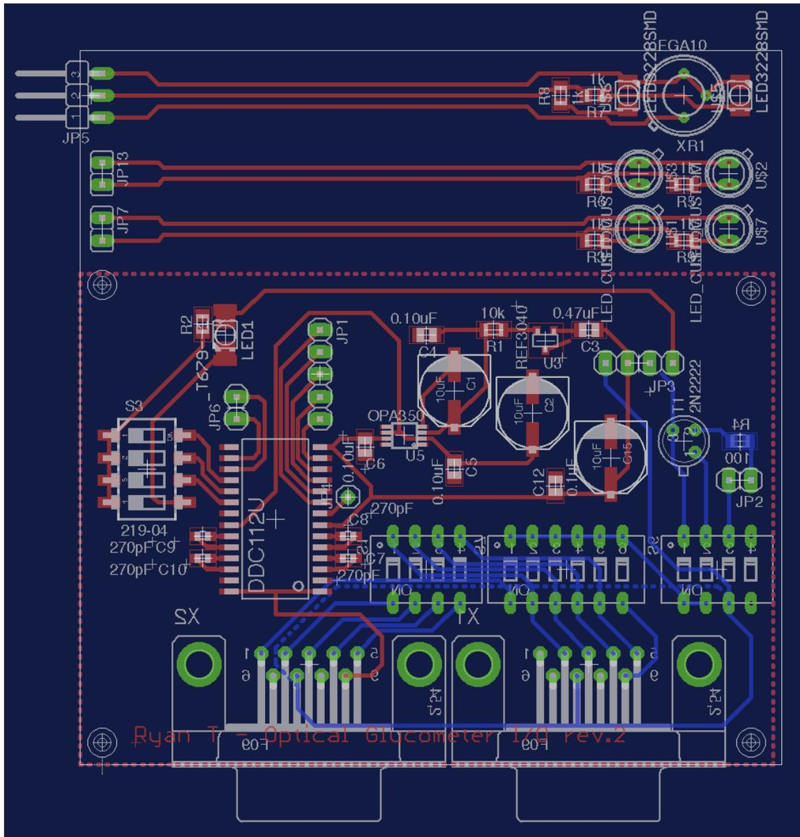
Figure 26: PCB with parts
