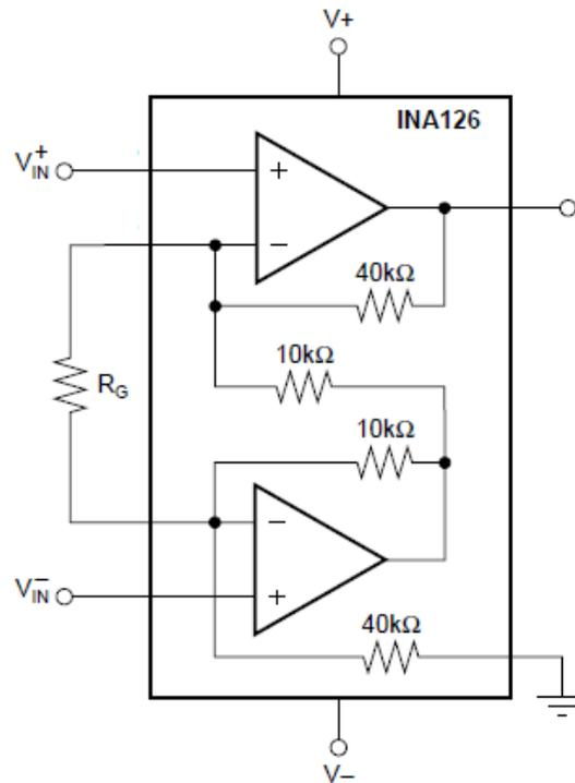
Figure 23: Instrumentation Amplifier
