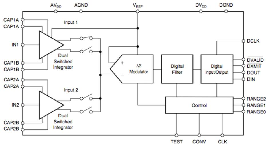
Figure 4: DDC112 Block Diagram.
