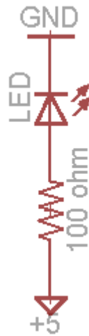
Figure 5: Schematic for the LED circuitry, each Red and IR LED would have a separate circuitry associated with it
