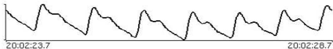
Figure 2 Pulsatile signal obtained when IR or red light is transmitted through the finger. Figure taken from Medical Electronics , Dr. Neil Townsend.
