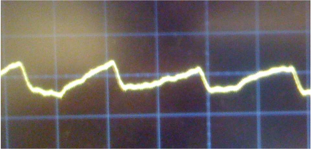
Figure 20: Oscilloscope reading from the IR LED (each division is 10 mV)
