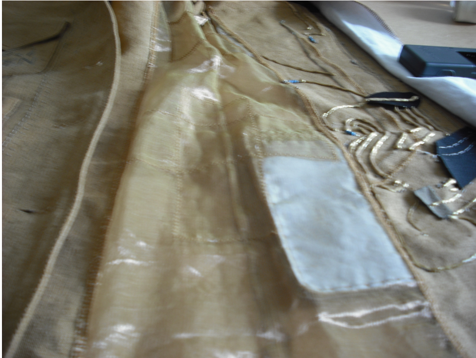
Figure 10. The inside of one side of the coat with the gold puffy fabric paint covering the circuit paths.
