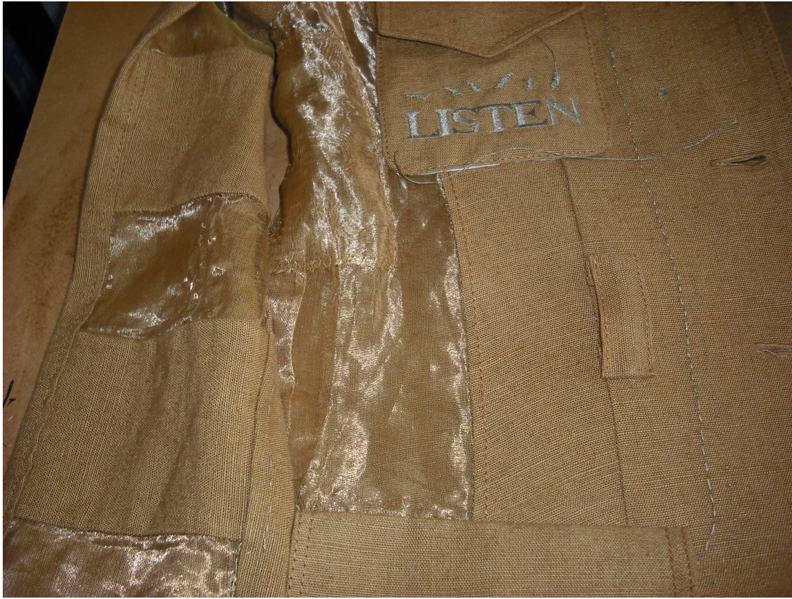
Figure 8. The embroidered sensor and a section of the sleeve sensor.
