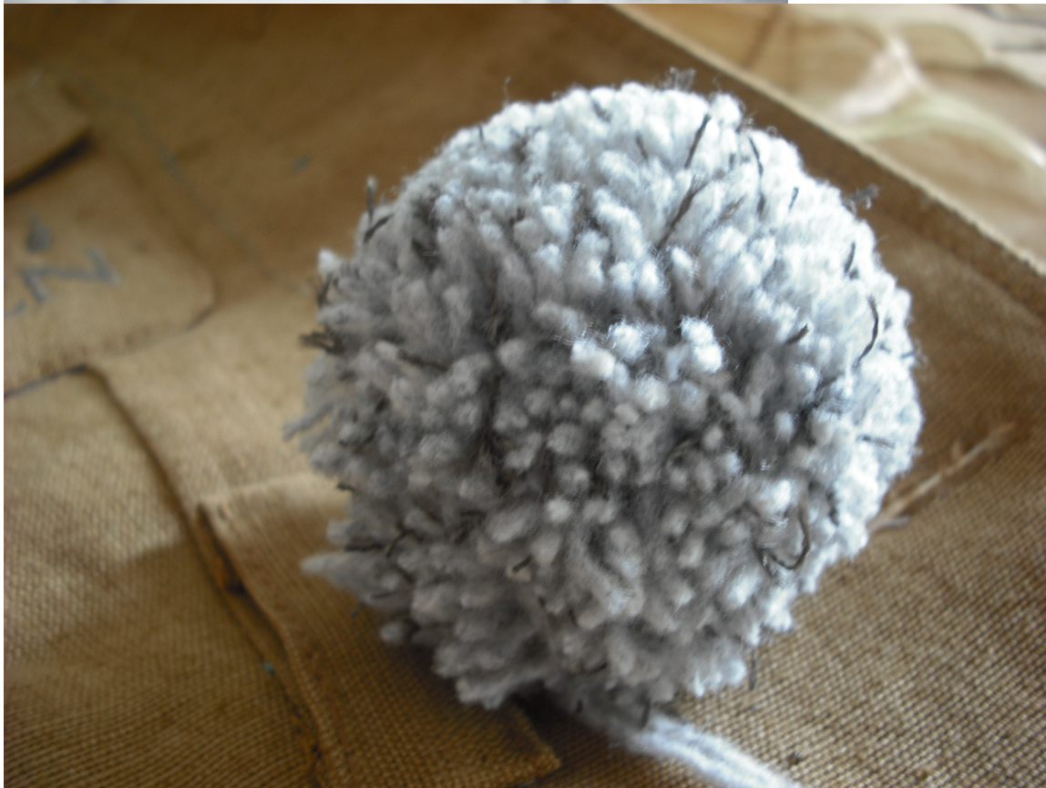
Figure 4. One of the conductive pom-poms I made. The thin silver thread is conductive.
