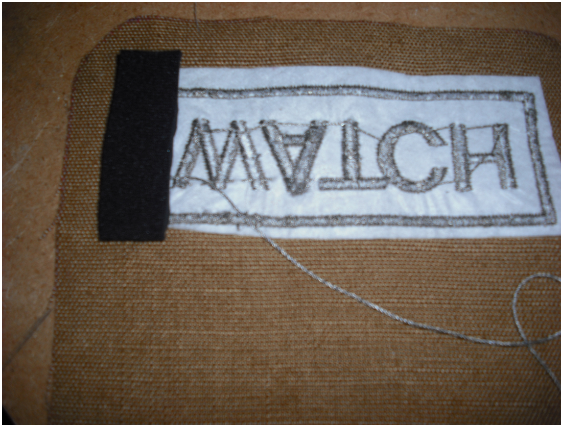
Figure 2. The soft circuit of the embroidered sensor is connected with conductive thread. In this photograph each letter of the word WATCH is connected to form the connections to an area that is designated the “power” part of the sensor. I used a small patch of neoprene to insulate the circuit path so that the ground circuit path could be sewn underneath it.
