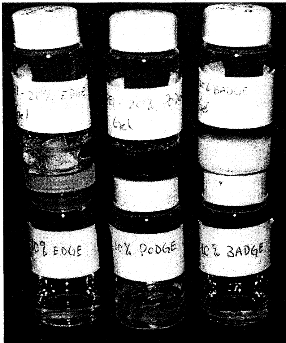
Figure 4.2 Photograph of 10% and 20% EDGE, PODGE and BADGE cross-linked BPEI gels. Distortions in the 20% EDGE and PODGE gels were caused by removal of samples for microscopic analyses and were not defects in gel structure. All gels made with same polymer concentration
