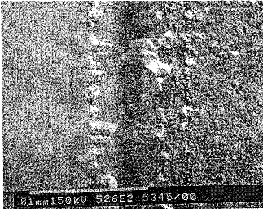
Figure 5.25. SEM image of CBN cutting tool showing wear on the rake face. ( V=268.8 m/min, f=0.1016 mm/rev).
