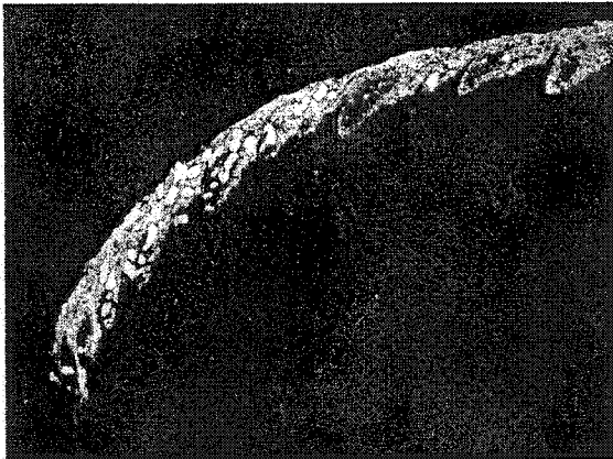
Figure 3.18-a. Micrograph of chip formed during cutting D2 with a honed cutting edge. (N=10000 RPM, ADOC =0.625 mm, f=0.0254 mm/tooth, 38 mm diameter high volume fraction CBN ball end mill).
