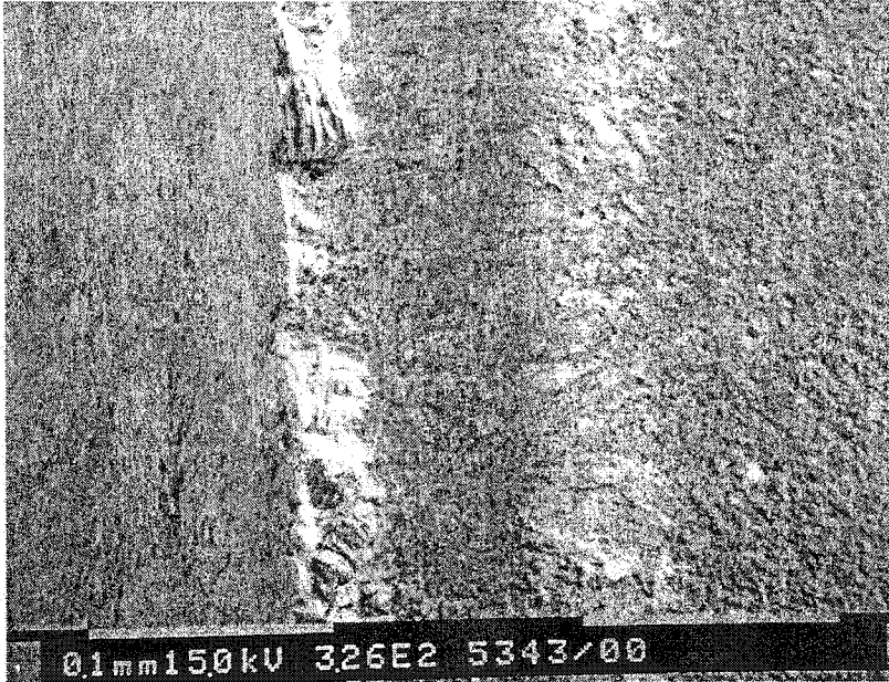
Figure 5.13. SEM image of the rake face of the cutting tool producing the chips in figure 5.5. ( V=55 m/min, f=0.1016 mm/rev).
