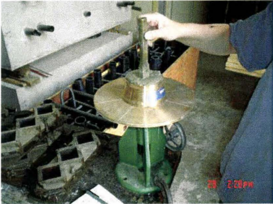
(b) Flow Test for Workability (before test)
