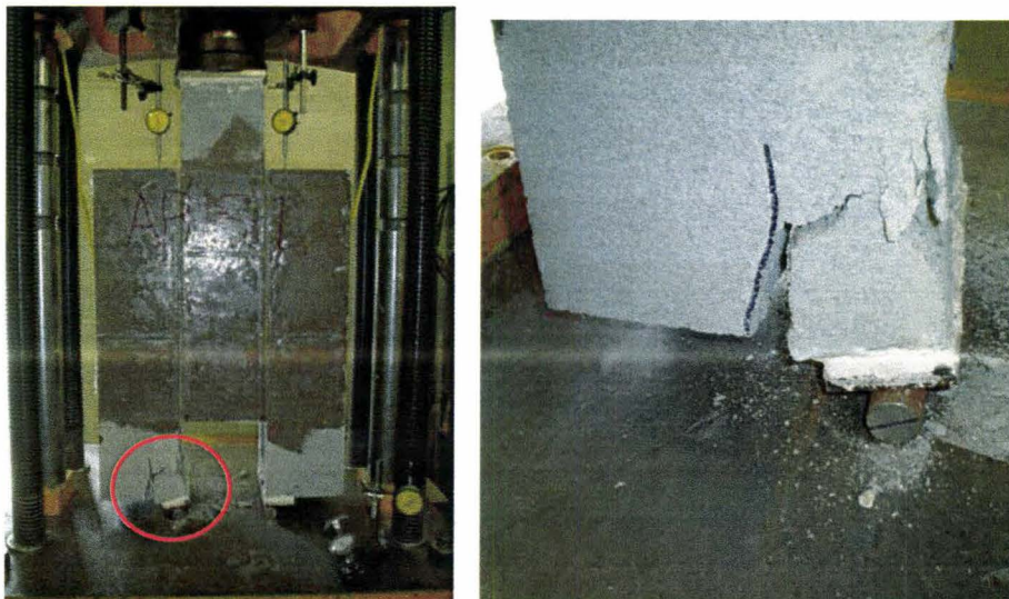
Figure 3.7 – Block Crushing at Lower Support Point of Specimen AR – 1.5 – 1
