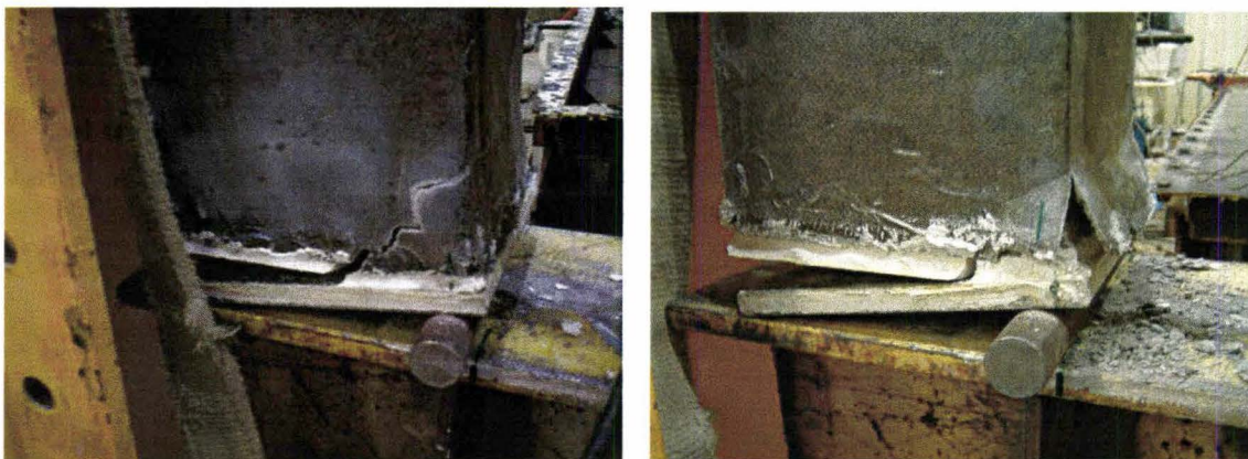
Figure 3.13 – Typical Block Crushing at Lower Support Point of Specimen AR-2.5
