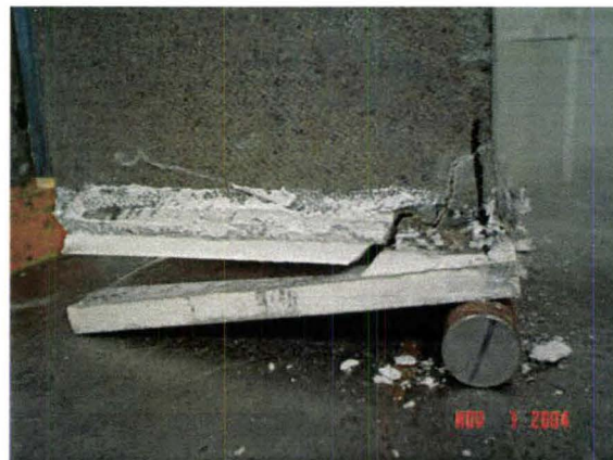
Figure 3.9 – Block Crushing at Lower Support Point of Specimen AR – 1.5 – 2
