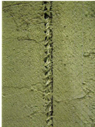
Figure 4.13 – Typical Fibre Damage (Tearing) of a Bed Joint Reinforced with 9.0 oz. Mesh at \pm 45^\circ
