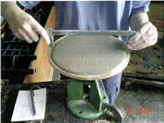
(c) Flow Test for Workability (after test)
