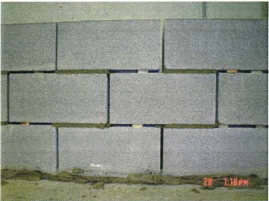
(c) 10 mm Plywood Strips Used as Spacers to Separate the Specimens
