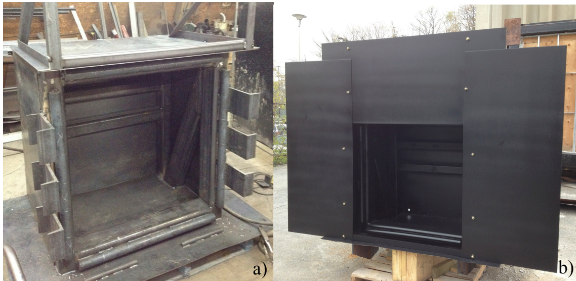
Figure 2.8: Blast Test-Frame; a) Without wing Walls, and b) With wing walls
