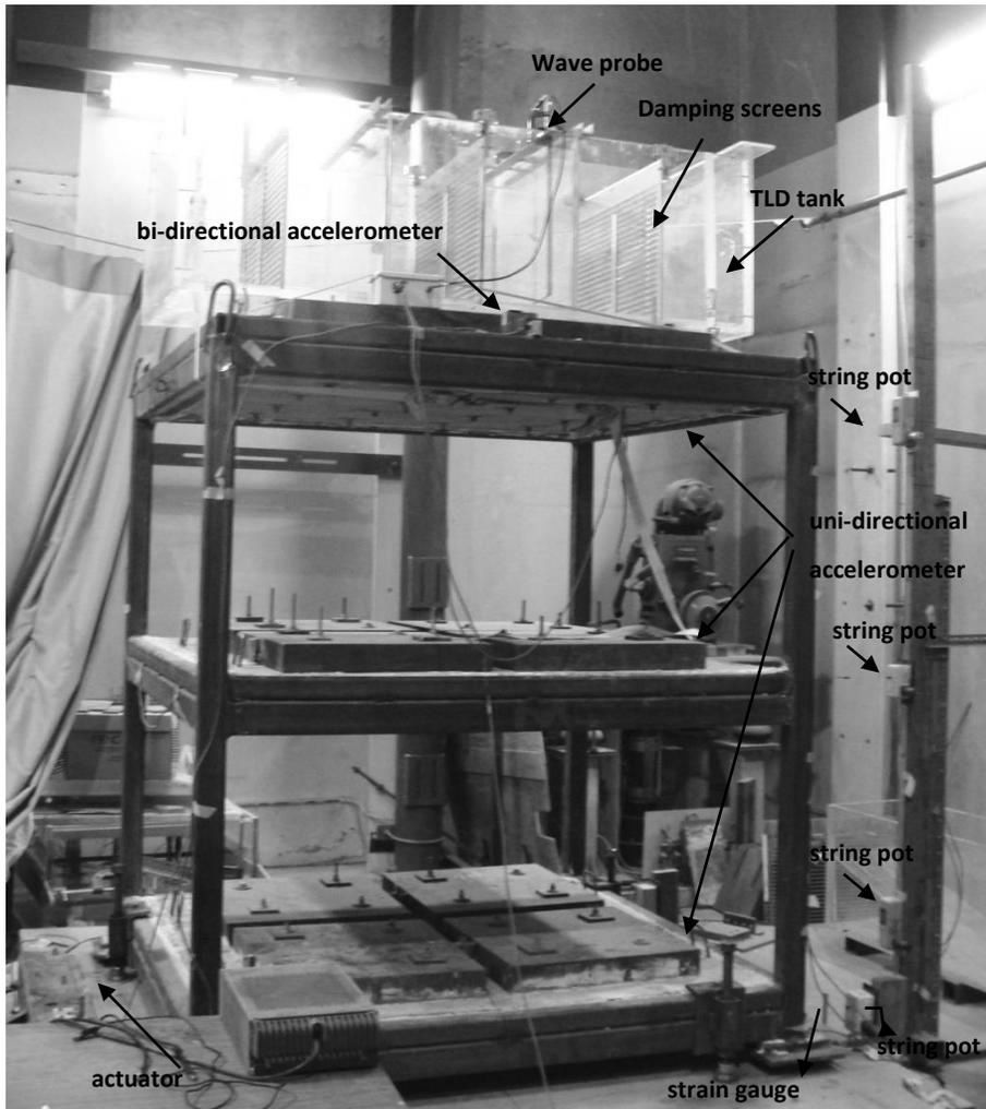
Figure 3-3 Photograph of shake table test setup
