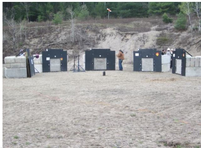
Figure A.2.4. Blast Test Bunkers Facing Charge
