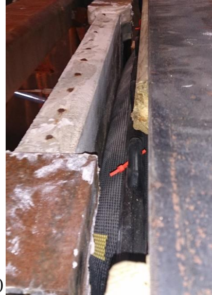
Figure A.3.1. Static Test Setup: a) Airbag; b) Airbag between Wall and Reaction Frame
