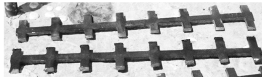
Figure 2.6. Steel Test Specimens (with connecting tabs)
