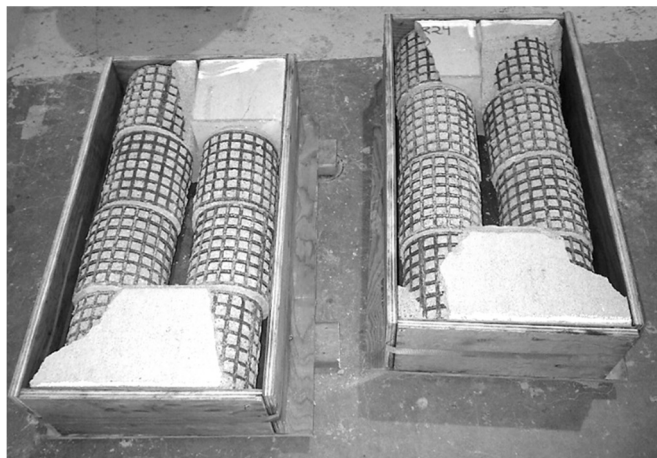
Figure 3.23. Tested SR Block Prisms Positioned in Forms in Preparation for Repair
