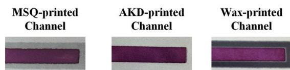
Fig. 2 Flow of dye solutions in various channels.
