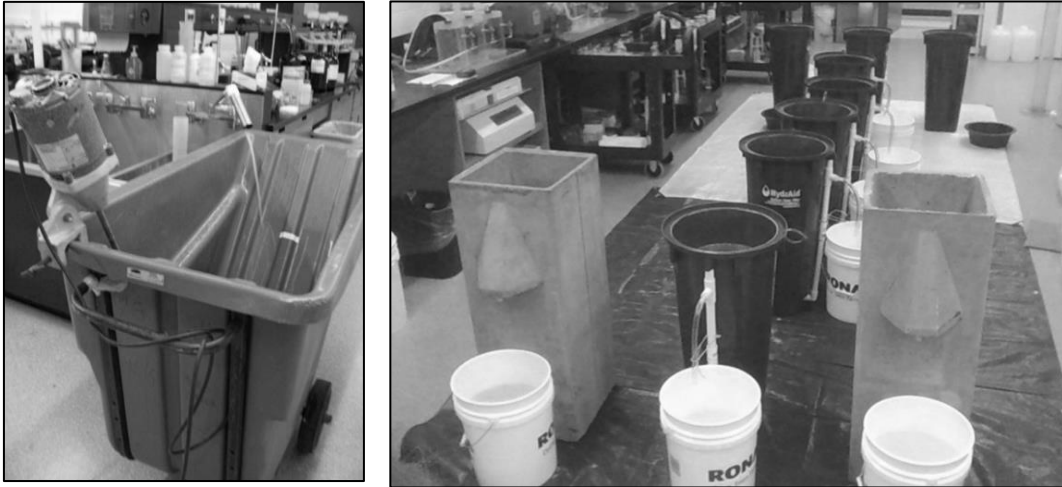
Figure B- 1 Bin for mixing influent water (left) and overview of lab set-up with all ten filters (right).
