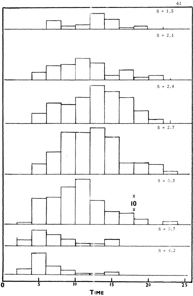
Fig. 13. The probability of droplet nucleation with time for magnesium salt. Method of detection: plane polarized light.
