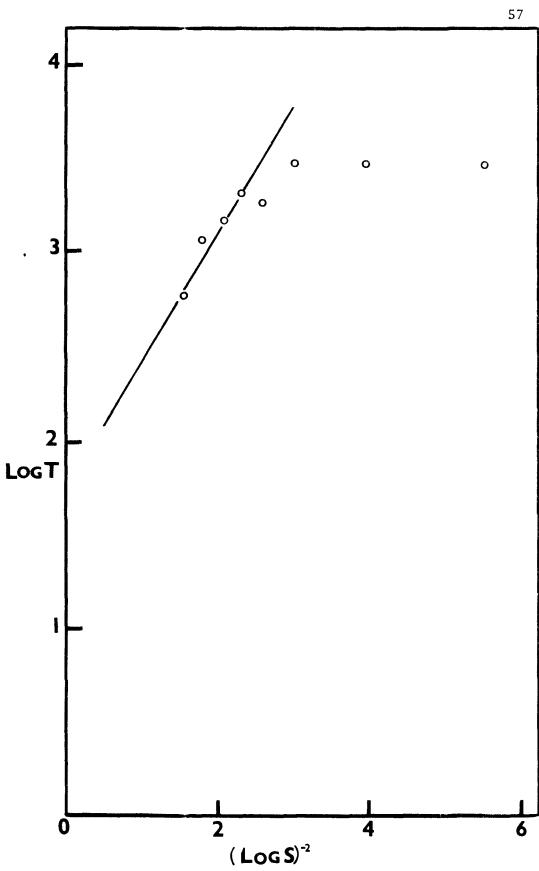
Fig. 11. The plot of  $\log J$  vs  $(1/\log S^2)$  for calcium salt.
