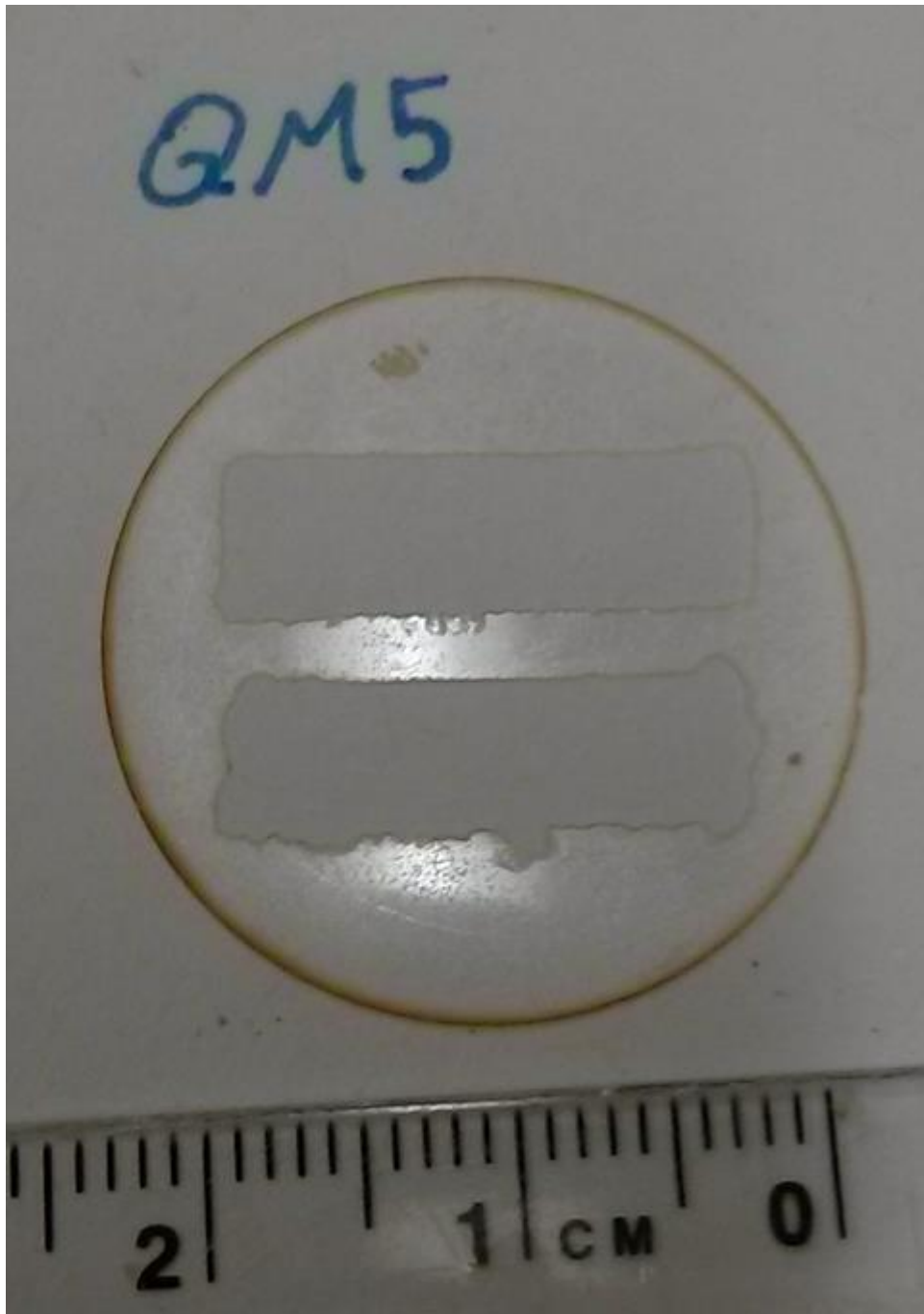
Figure 6-6: QM5: The quartz mask used for back RIE of QSU8_17, after its retirement This RIE thins down the quartz by 96 \mu\text{m} , from an initial 104 \mu\text{m} to only 7.6 \mu\text{m} thickness (determined by optical profilometry). Following the thinning, the sample appears as shown in Figure 6-7.
