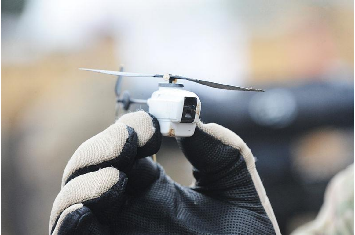
Figure 1-2: The 16 g Black Hornet UAV currently operated in Afghanistan by the British Army [7]
