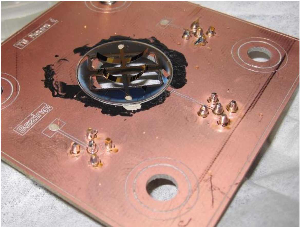
Figure 6-12: QSU8_17 mounted on its PCB for testing
