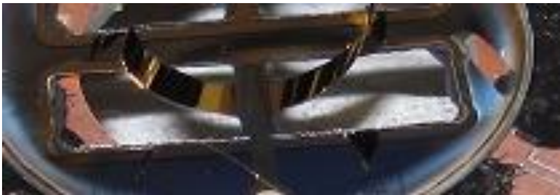
Figure 8-13: The tested wings twisted out of the plane of perfectly cylindrical arcs
