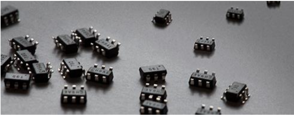
Figure 4-28: Atmel's ATtiny4 microcontroller is only 2 mm by 2 mm by 0.5 mm including the package, and uses only 0.4 mW of power when active at 1 MHz [46]
