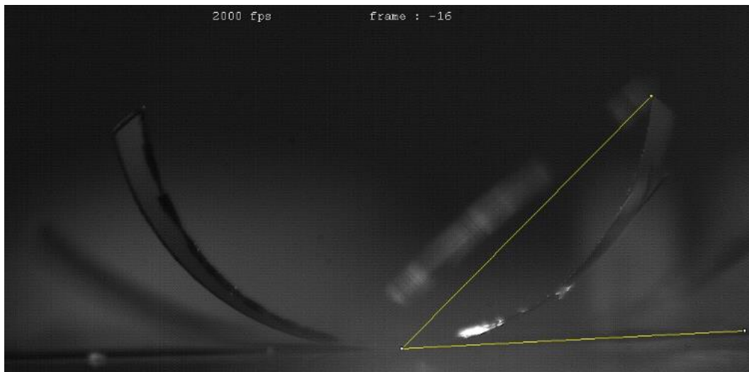
Figure 7-1: Measuring the wing angle using ImageJ
