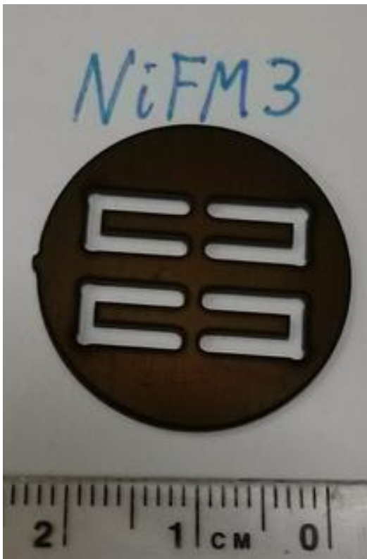
Figure 6-10: NiFM3, the Nickel Front Mask used for RIE wing release of QSU8_17
