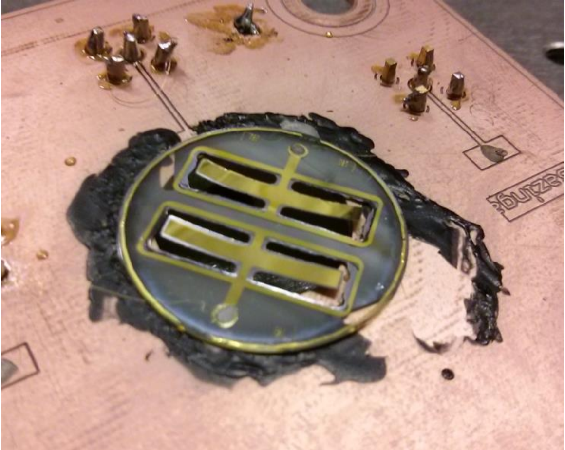
Figure 8-5: After almost continuous testing for 2 years and tirelessly flapping over 5 billion times, QSU8_17 settles into retirement in June 2013 after months at vacuum pressures lower than 1e-8 atm were too much for its built-in curvature
