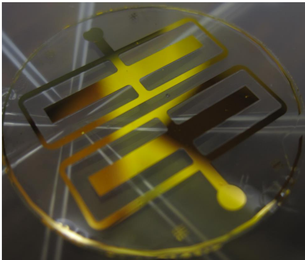
Appendix Figure R-4: Sample QSU8_14 after SU-8 patterning
