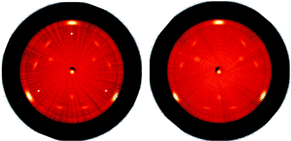
(a) (111) pole figure of ZnTe epitaxially grown on sapphire. (b) (111) pole figure ZnTe after liftoff on polysulphone carrier.
