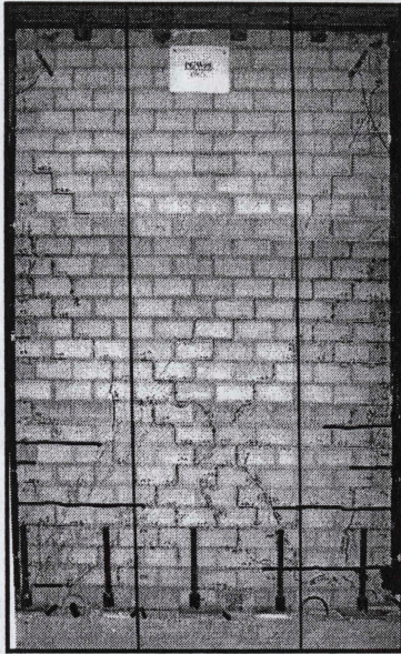
(a) New cracks during 1.50 mm, 2.00 mm and 2.50 mm disp. cycle
