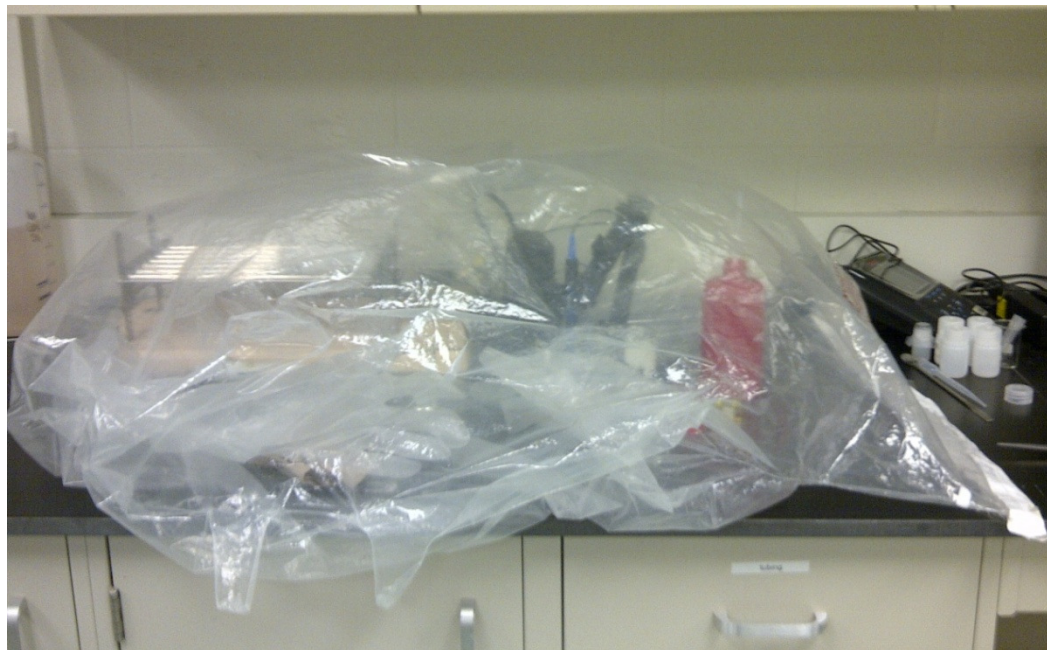
Figure 3.2: Glove bag with N_2 to mitigate contamination
