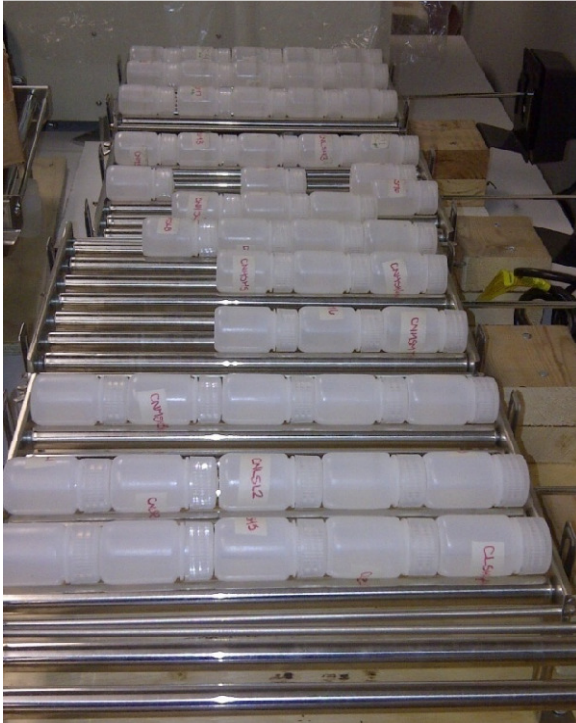
Figure 3.4: Rollers used for continuous mixing of samples
