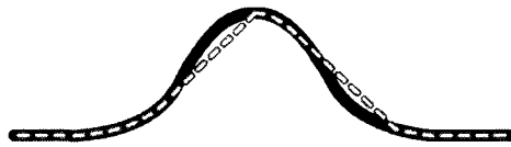
Figure 4.1: Effects of limiting slew rates
